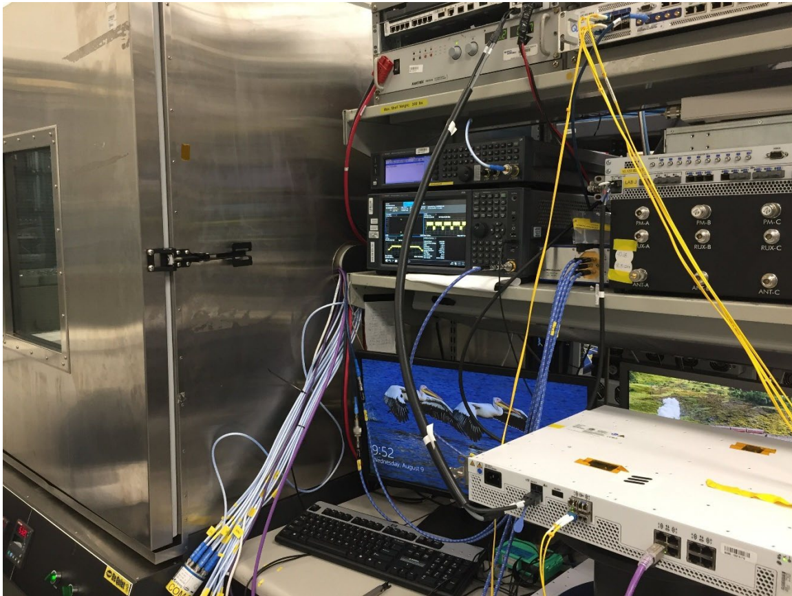
Figure 5: Conducted test setup (Frequency Stability)
