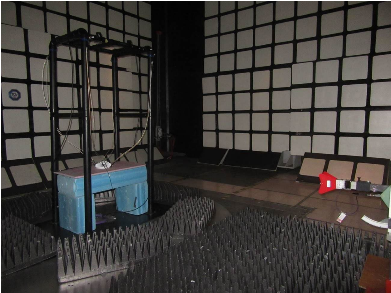
Figure 2: Radiated Test setup (frequency above 1000MHz)
