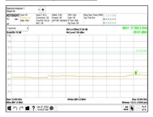
Antenna A - Modulation NR80: QPSK (NC) - Carrier Bandwidth NR80.0+NR80.0 MHz - Channel Position B - Band 4 - Range 18000 to 39800 MHz
