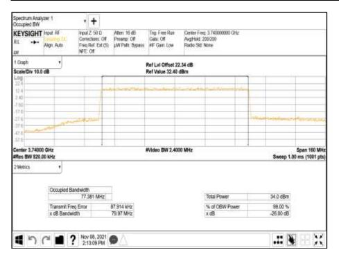
Antenna A - Modulation NR: QPSK - LTE Carrier Bandwidth NR: 100.0 MHz - Channel Position B
