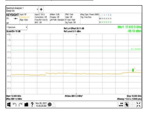
Antenna A - Modulation NR20: QPSK - Carrier Bandwidth 20+20+20+20+20+20 MHz - Channel Position B - Band 4 - Range 18000 to 38900 MHz
