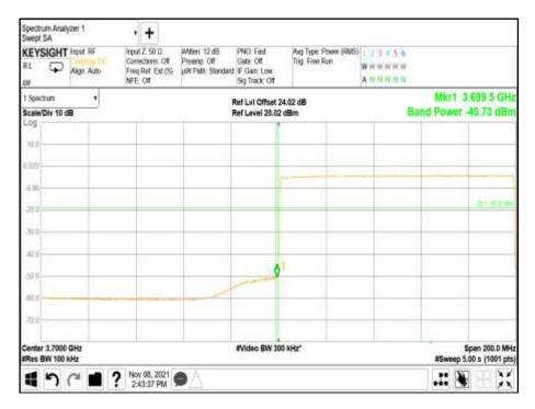
Antenna Port A - Modulation NR: QPSK - Carrier Bandwidth NR: 100.0 MHz - Channel Position T
