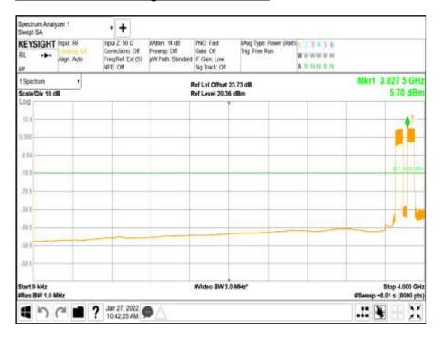
Antenna A - Modulation NR80: QPSK (NC) - Carrier Bandwidth NR80.0+NR80.0 MHz - Channel Position B - Band 2 - Range 4000 to 12000 MHz
