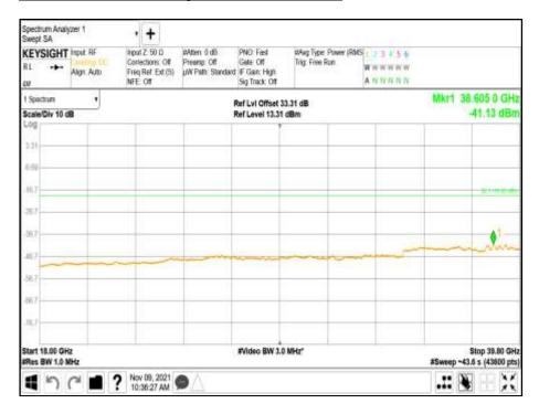
Limit The power of any emission outside of the authorized operating frequency ranges must be attenuated below the transmitting power (P) by a factor of at least 43 + 10 log(P) db.
