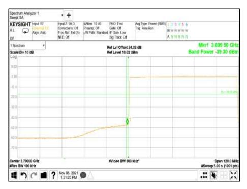
Antenna Port A - Modulation NR: QPSK - Carrier Bandwidth NR: 60.0 MHz - Channel Position T
