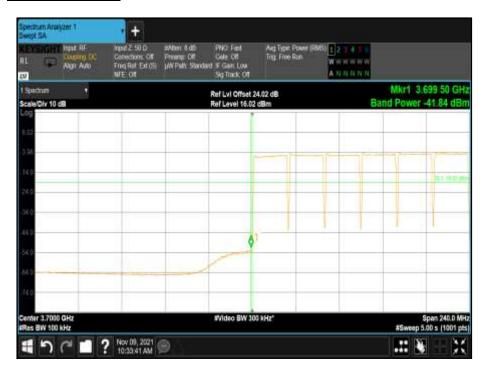
Antenna Port A - Modulation NR20: QPSK - Carrier Bandwidth 20+20+20+20+20+20 MHz - Channel Position T
