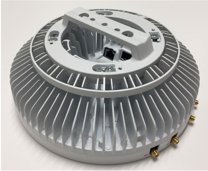
Figure 2: The EUT with four external RF ports, Dot 41Kr B77D
