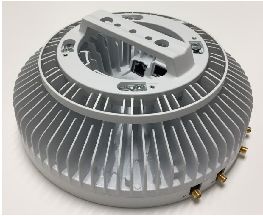
Figure 2: The EUT with four external RF ports, Dot 4469 B77D
