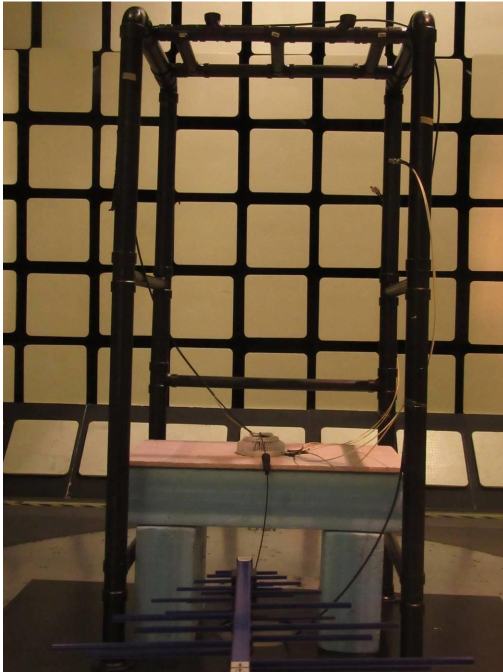
Figure 41: Setup for RE tests at 30 MHz to 1 GHz (Configuration 1)
