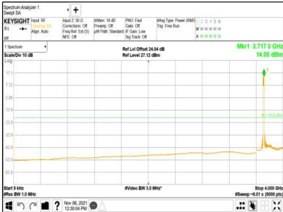
Antenna A - Modulation NR: QPSK - Carrier Bandwidth 20.0 MHz - Channel Position B - Band 2 - Range 4000 to 12000 MHz
