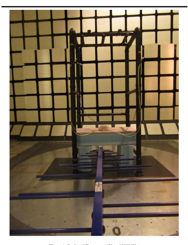
Figure 1: Radiated Test setup (30 to 1000MHz)
