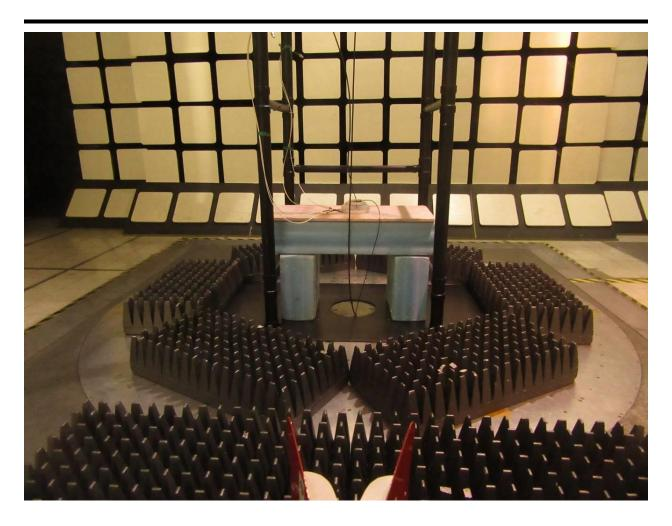
Figure 2: Radiated Test setup (frequency above 1000MHz)
