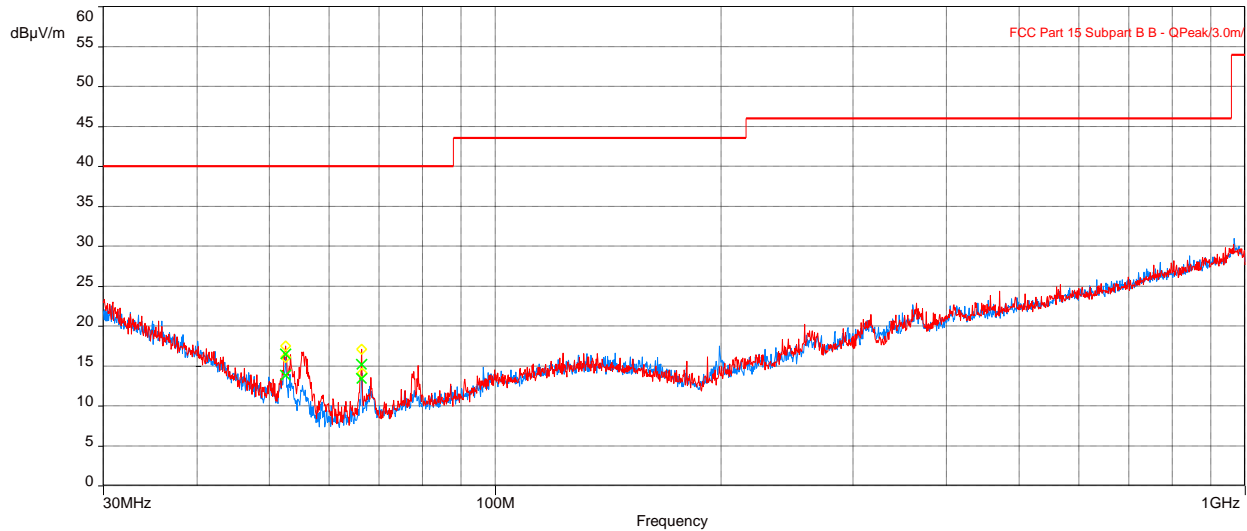
Figure 16: Plot of RE at 3 m – 30 to 1000 MHz (LTE – Middle channel)
