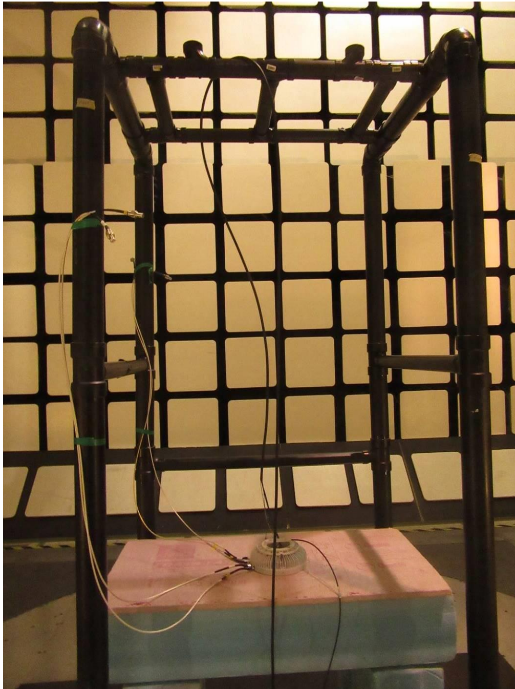
Figure 49: Setup for RE tests - Close up (Configuration 2)
