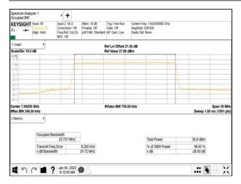
Antenna A - Modulation NR: QPSK - LTE Carrier Bandwidth NR: 30.0 MHz - Channel Position B
