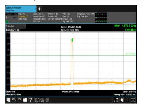
Antenna A - Modulation NR25+NR25: QPSK - Carrier Bandwidth 25+25 MHz - Channel Position B - Band 2 - Range 4000 to 12000 MHz
