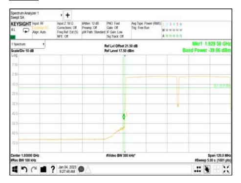
Antenna Port A A - Modulation NR30+NR30: QPSK - Carrier Bandwidth 30+30 MHz - Channel Position T
