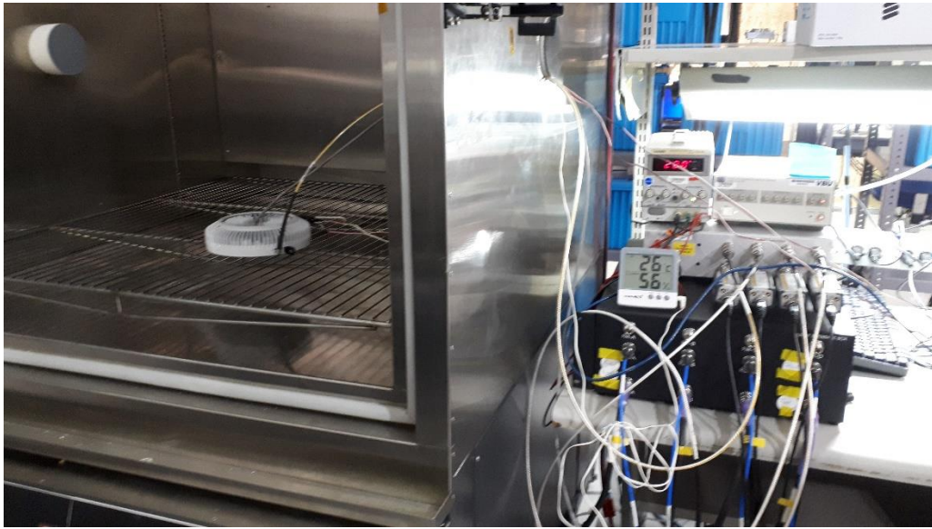
Figure 4: EUT test fixture in a thermal test chamber
