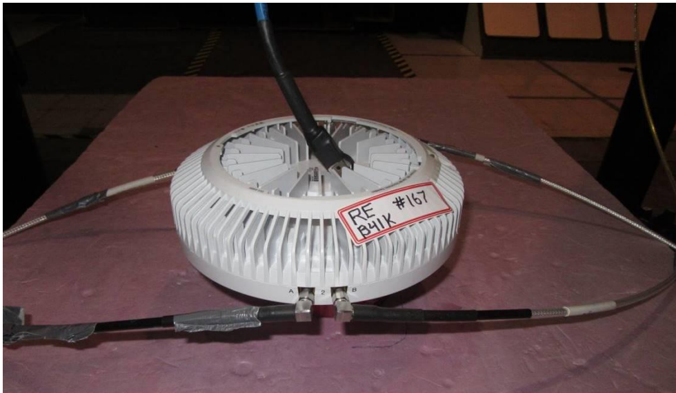
Figure 1: The EUT with four external RF ports
