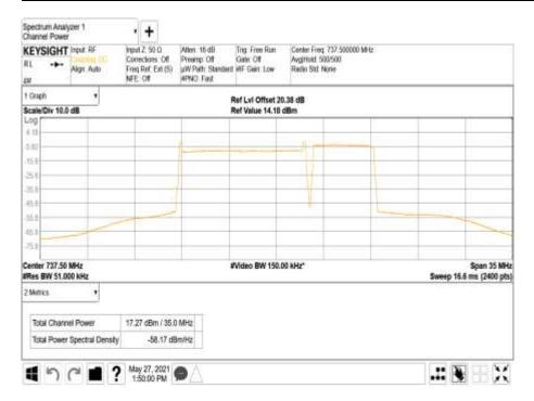
Antenna B - Modulation LTE + NR: QPSK - Carrier Bandwidth 10.0+5 MHz - Channel Position B
