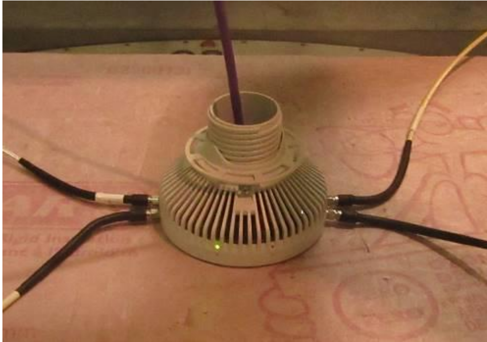
Figure 2: The EUT with External antenna (DOT 2282)
