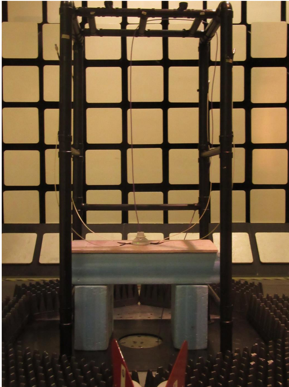
Figure 41: Setup for RE tests for above 1 GHz (Tx mode – Dot 2282)
