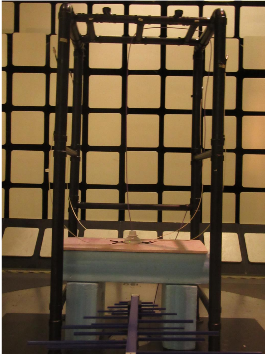
Figure 40: Setup for RE tests at 30 MHz to 1 GHz (Tx mode – Dot 2282)
