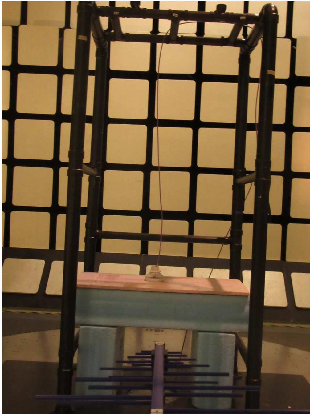
Figure 42: Setup for RE tests at 30 MHz to 1 GHz (Rx mode – Dot 2272)
