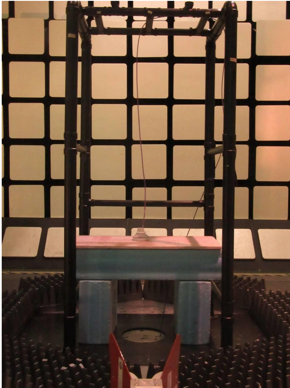
Figure 43: Setup for RE tests for above 1 GHz (Rx mode – Dot 2272)
