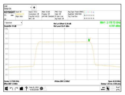
Antenna Port A Carrier Power - Modulation NR: QPSK - Carrier Bandwidth 5.0 MHz - Channel Position T
