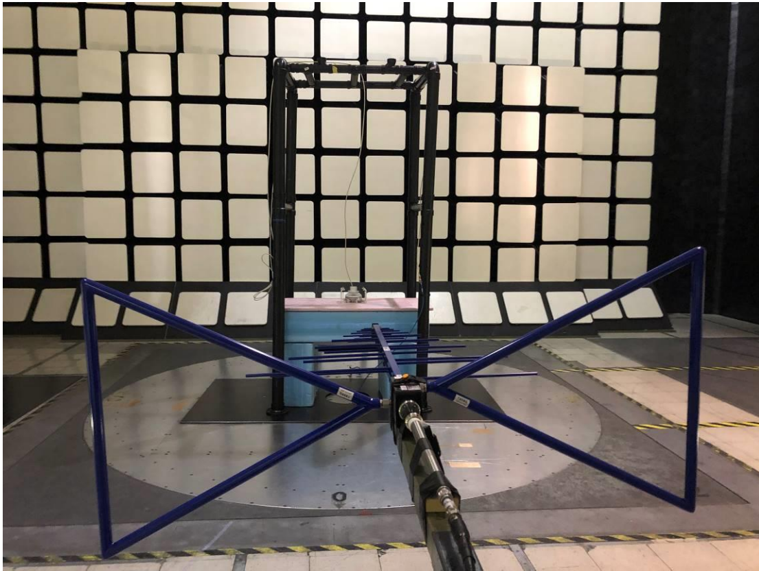
Figure 54: EUT Setup for RE tests at 30 MHz to 1 GHz
