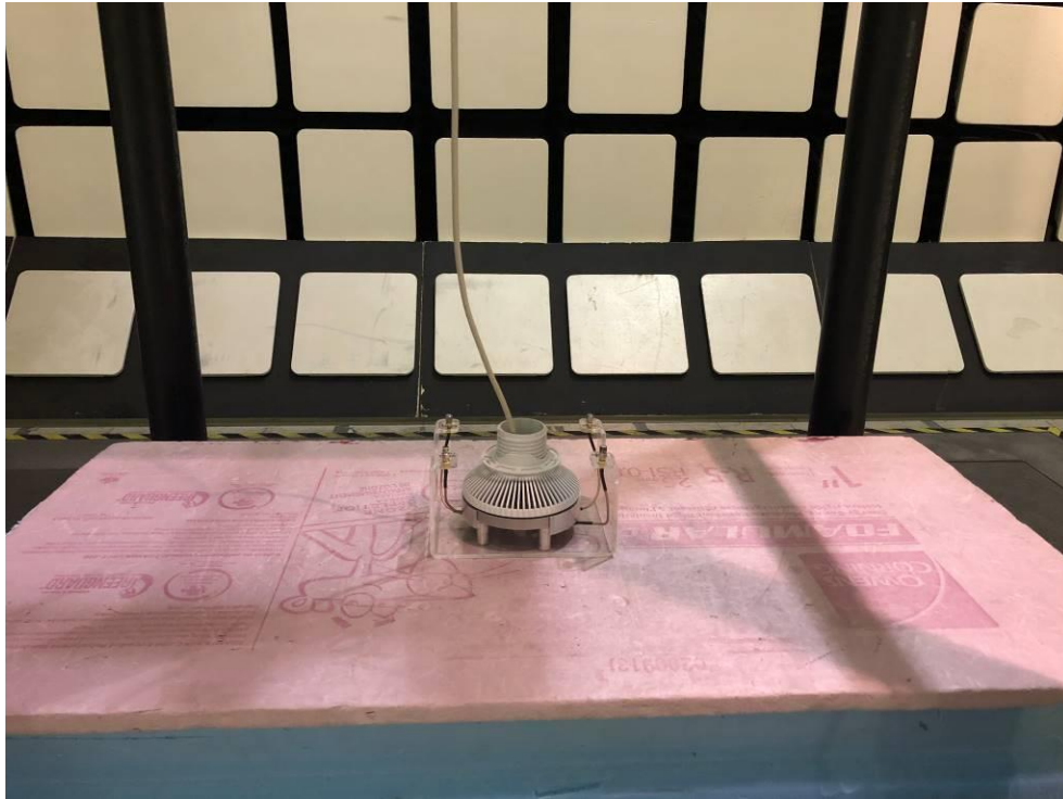
Figure 53: EUT Setup for RE tests (Closeup)
