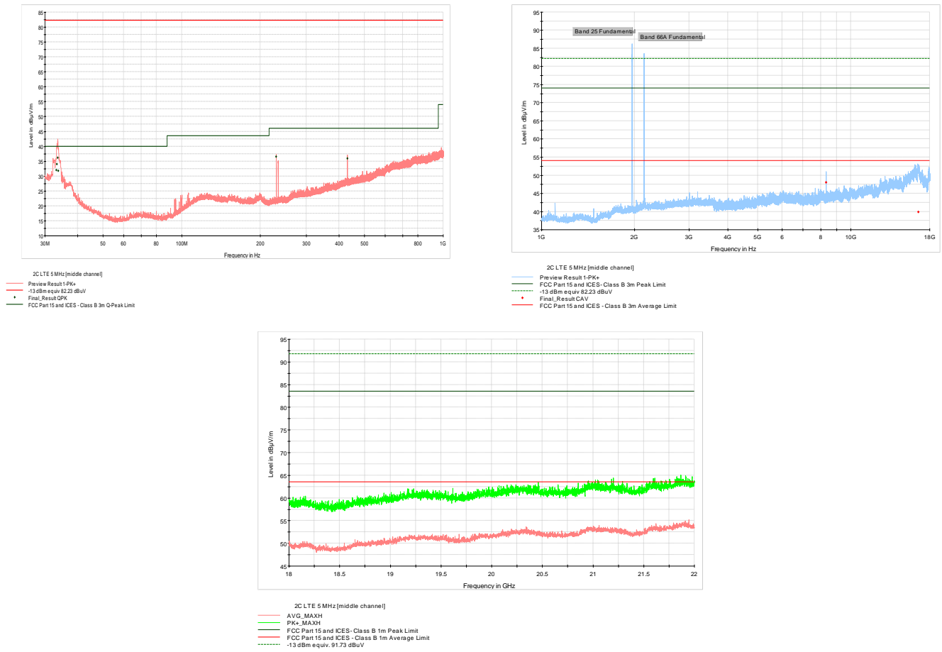
Figure 7.1-5: Radiated emissions spectral plot (30 to 22000 MHz) – Dual carrier 5 MHz channel [middle][LTE]
