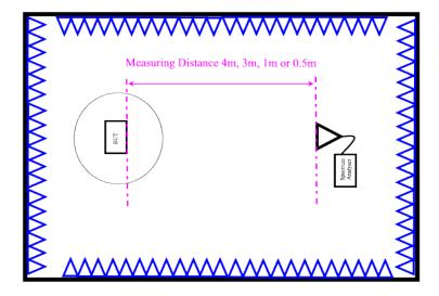
1 GHz – 40 GHz the measuring distance was 4m.
