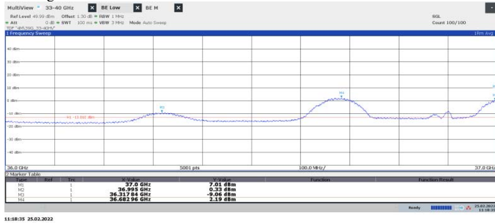
Diagram 2.7c: Pre scan 36 – 37 GHz, Symbolic name: BL2 max50 , EIRP Horizontal polarization See diagram 2.7e for TRP result
