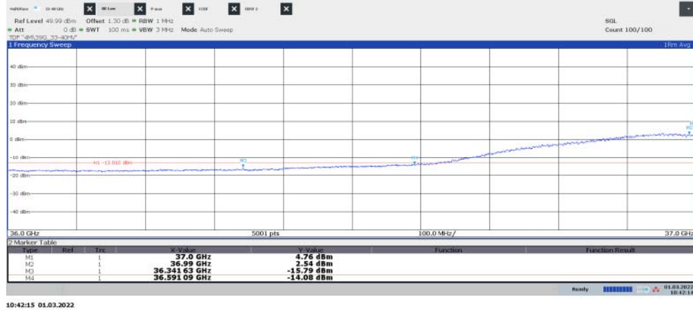
Diagram 2.33d: Pre scan 36 – 37 GHz, Symbolic name: BL8 100 , EIRP Vertical polarization
