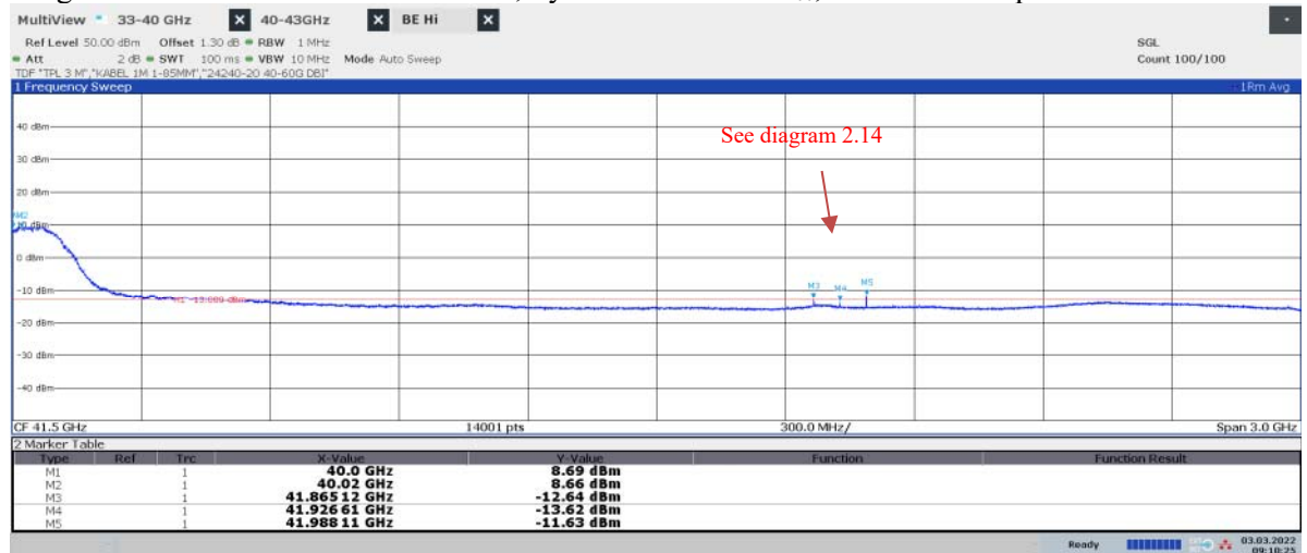
Diagram 2.17bd: Pre scan 40 – 43 GHz, Symbolic name: TH 200 , EIRP Vertical polarization
