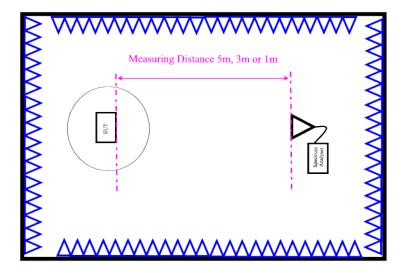
1 GHz – 40 GHz the measuring distance was 5m.
