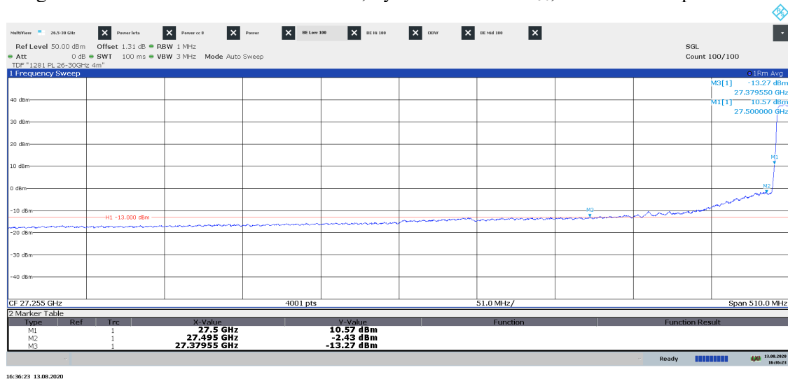
Diagram 2.7d: Pre scan 27.00 – 27.51 GHz, Symbolic name: BL 50 , EIRP Vertical polarization
