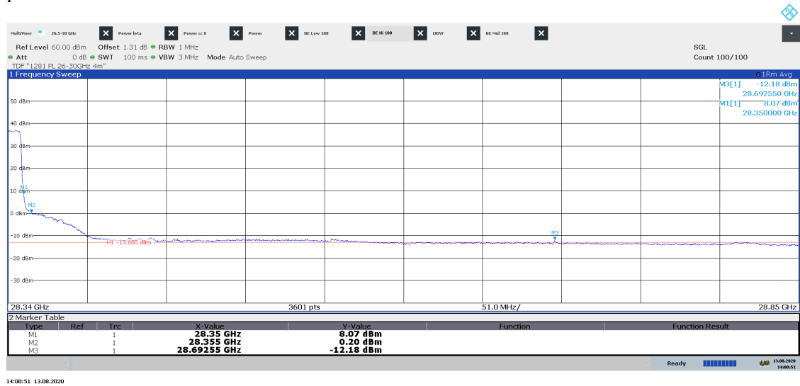
Diagram 2.12c: Pre scan 28.34 – 28.85 GHz, Symbolic name: TH 50 , EIRP Horizontal polarization
