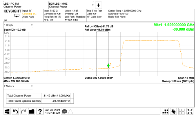
Figure 8.5-50: Conducted band edge emission at 1929 MHz, 5 MHz channel single-carrier operation (RBW = 1 MHz)
