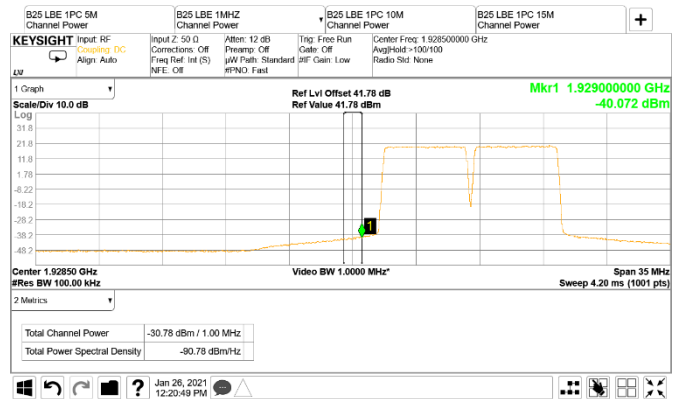
Figure 8.5-98: Conducted band edge emission at 1929 MHz, 5 MHz channel two-carrier LTE + NR operation (RBW = 1 MHz)
