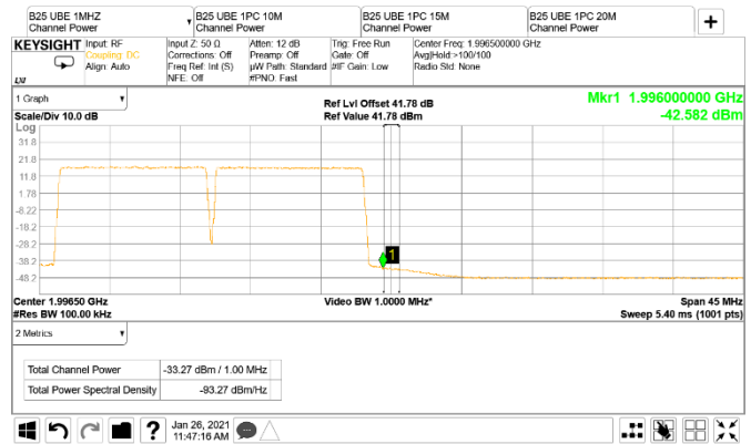
Figure 8.5-72: Conducted band edge emission at 1996 MHz, 10 MHz channel two-carrier operation (RBW = 1 MHz)
