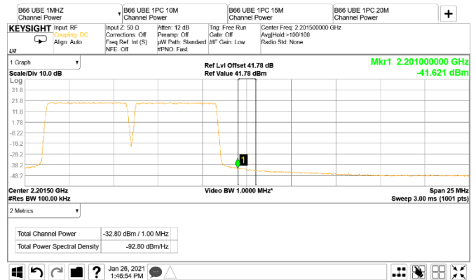
Figure 8.3-100: Conducted band edge emission at 2201 MHz, 5 MHz channel two-carrier LTE + NR operation (RBW = 1 MHz)
