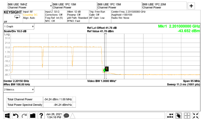
Figure 8.3-92: Conducted band edge emission at 2201 MHz, 15 MHz channel tree-carrier operation (RBW = 1 MHz)
