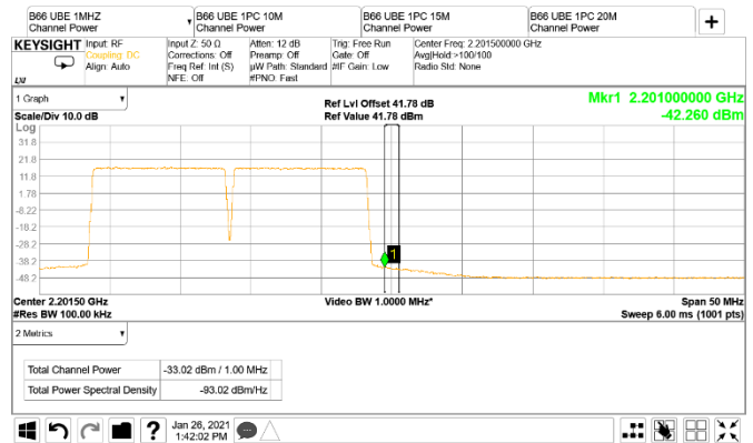
Figure 8.3-72: Conducted band edge emission at 2201 MHz, 10 MHz channel two-carrier operation (RBW = 1 MHz)
