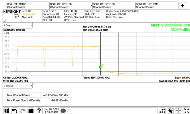
Figure 8.3-87: Conducted band edge emission at 2200 MHz, 10 MHz channel tree-carrier operation (RBW = 1% of EBW)
