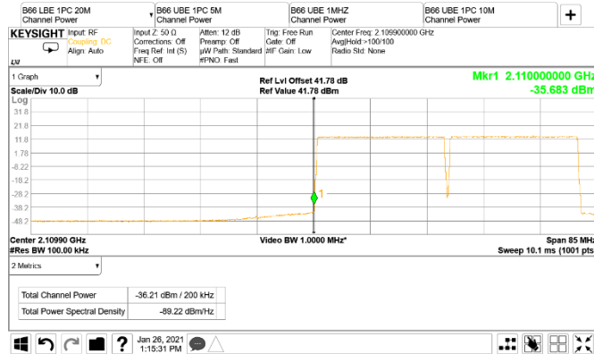
Figure 8.3-77: Conducted band edge emission at 2110 MHz, 20 MHz channel two-carrier operation (RBW = 1% of EBW)
