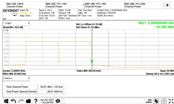
Figure 8.3-71: Conducted band edge emission at 2200 MHz, 10 MHz channel two-carrier operation (RBW = 1% of EBW)
