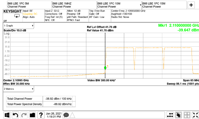
Figure 8.3-85: Conducted band edge emission at 2110 MHz, 10 MHz channel tree-carrier operation (RBW = 1% of EBW)
