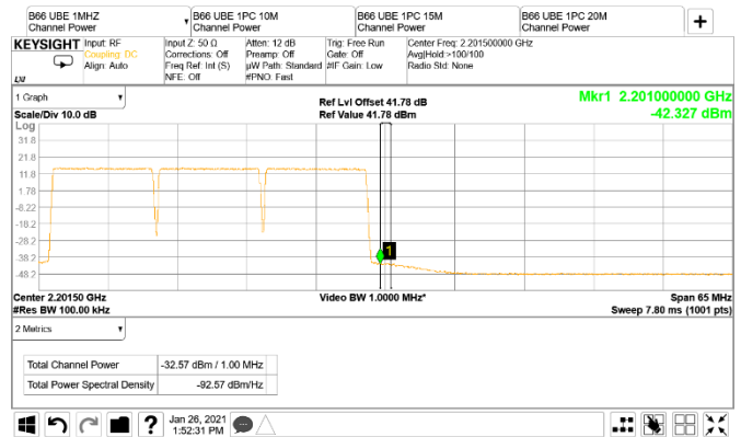
Figure 8.3-88: Conducted band edge emission at 2201 MHz, 10 MHz channel tree-carrier operation (RBW = 1 MHz)
