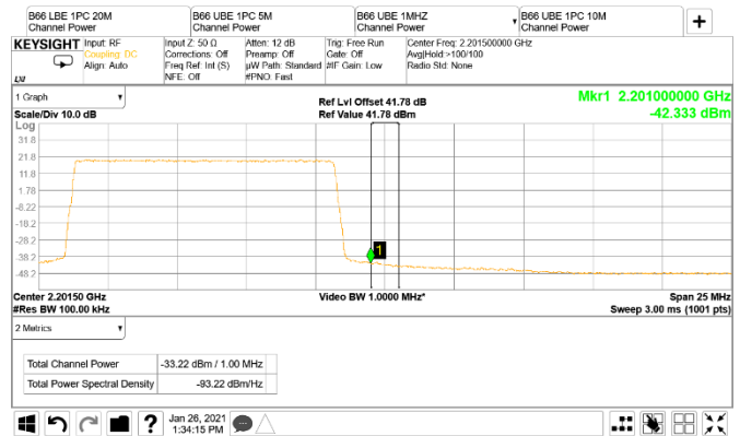
Figure 8.3-56: Conducted band edge emission at 2201 MHz, 10 MHz channel single-carrier operation (RBW = 1 MHz)
