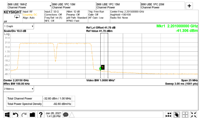
Figure 8.3-68: Conducted band edge emission at 2201 MHz, 5 MHz channel two-carrier operation (RBW = 1 MHz)
