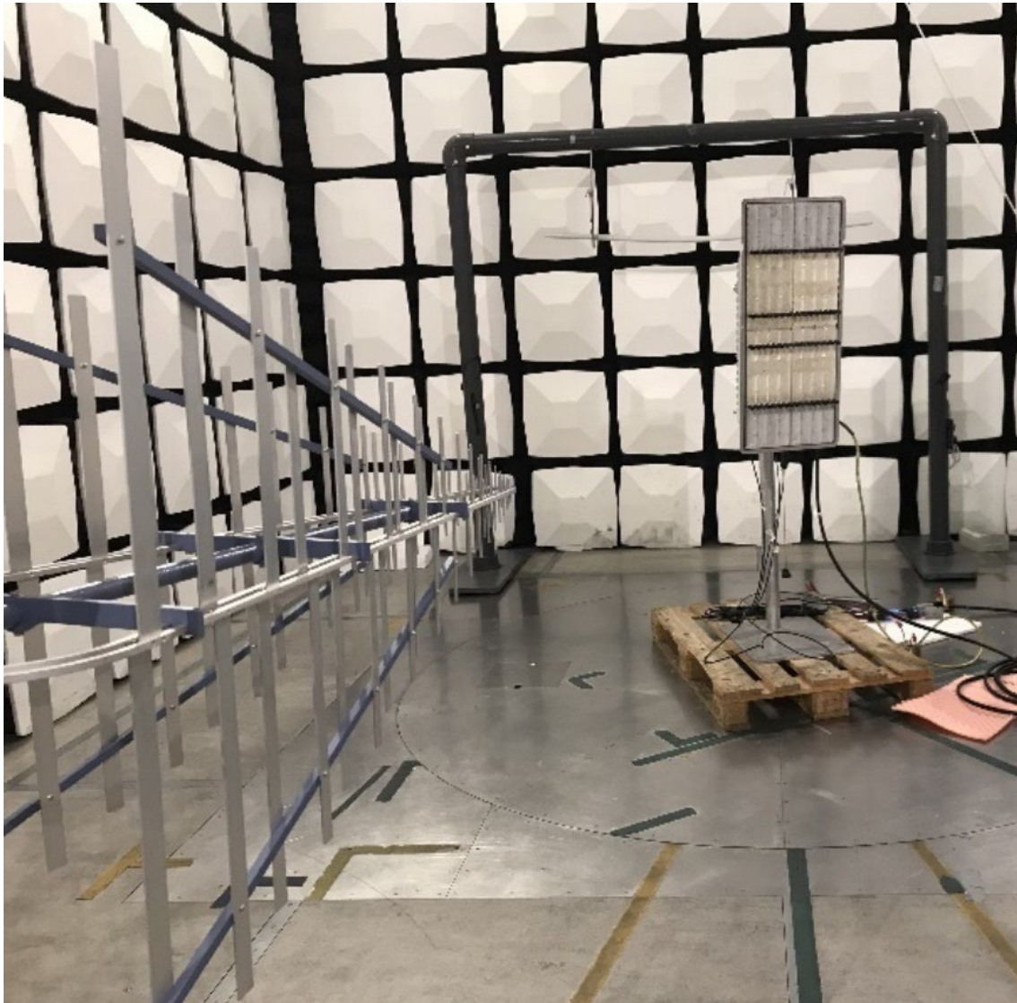
Photo of the test set-up for radiated emission 30 – 1000 MHz
