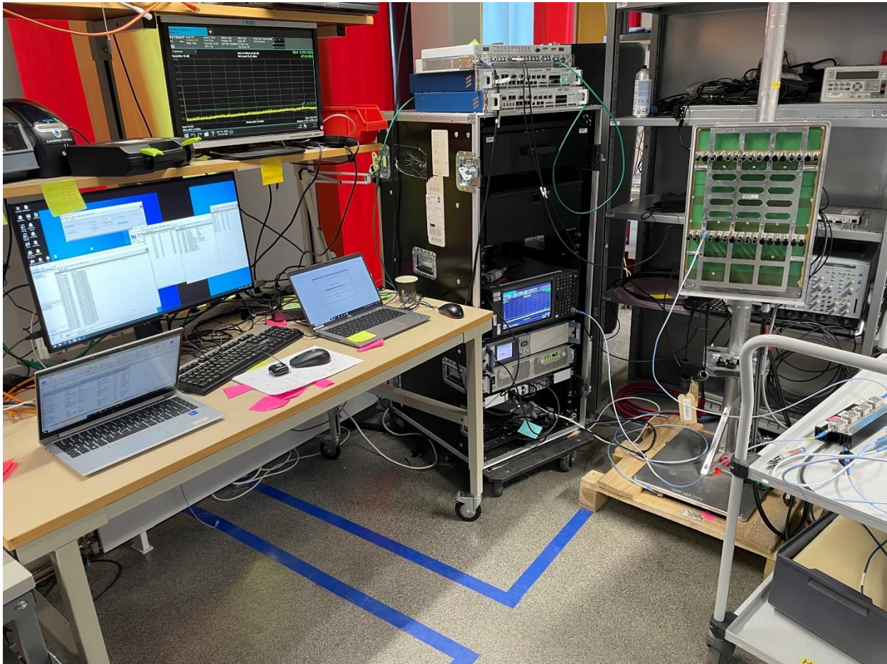
Conducted Lab Testing - Band Edge, Conducted Emissions
