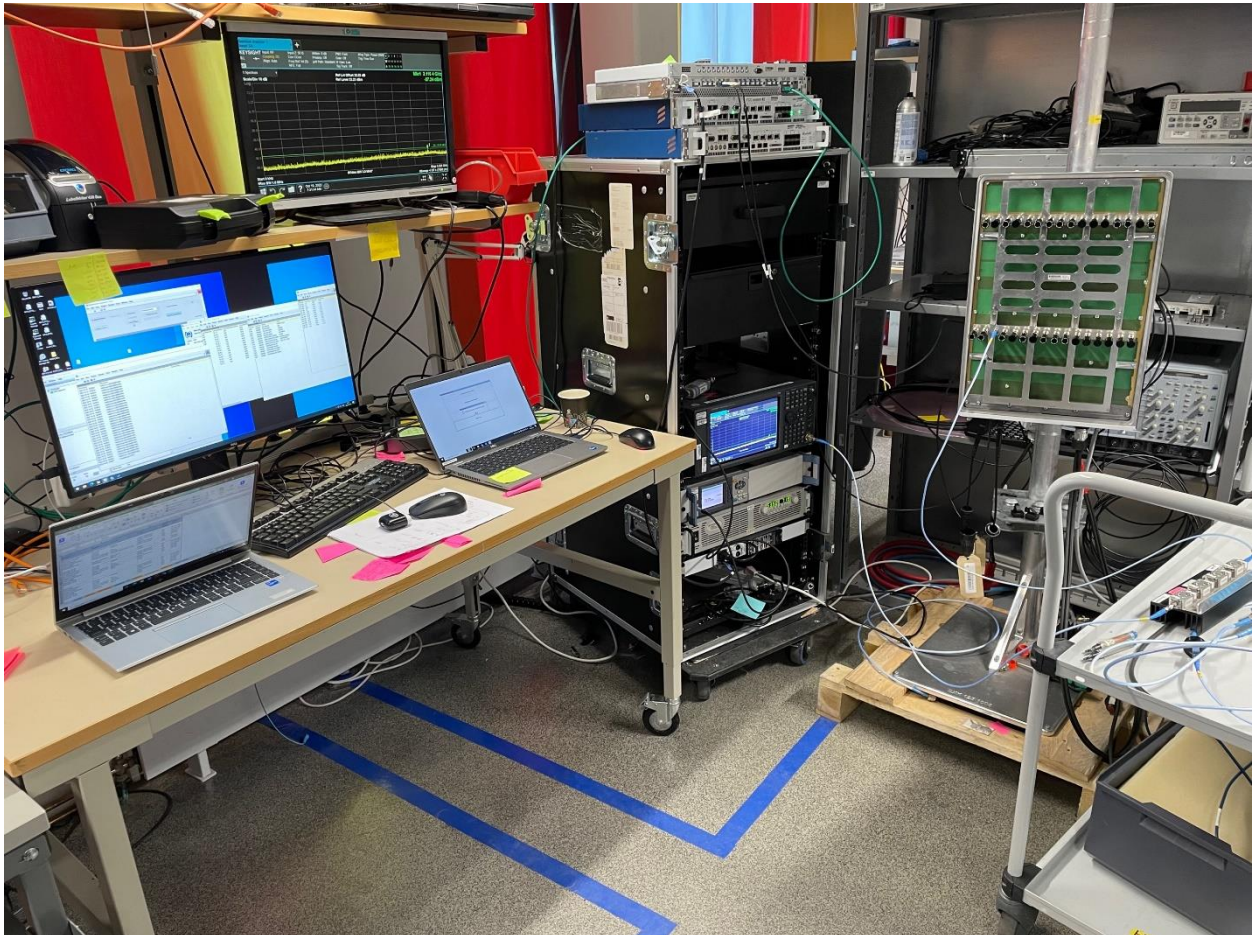
Conducted Lab Testing - Band Edge, Conducted Emissions
