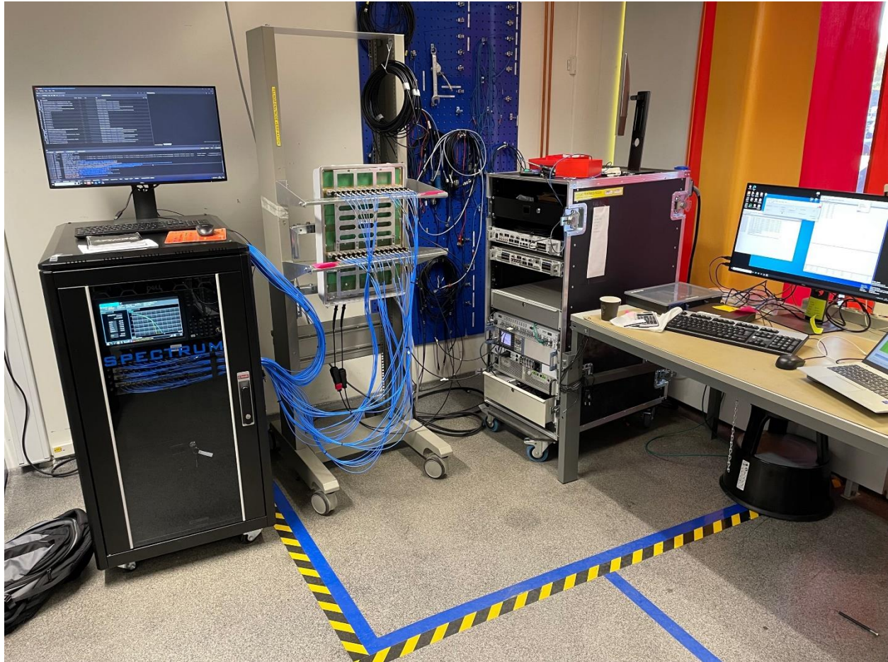
Conducted Test Set Up, Power, PSD, PAR, Occupied Bandwidth
