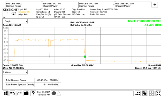
Figure 8.2-75: Conducted band edge emission at 2200 MHz, 15 MHz channel two-carrier operation (RBW = 1% of EBW)
