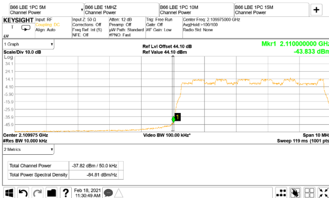
Figure 8.2-49: Conducted band edge emission at 2110 MHz, 5 MHz channel single-carrier operation (RBW = 1% of EBW)
