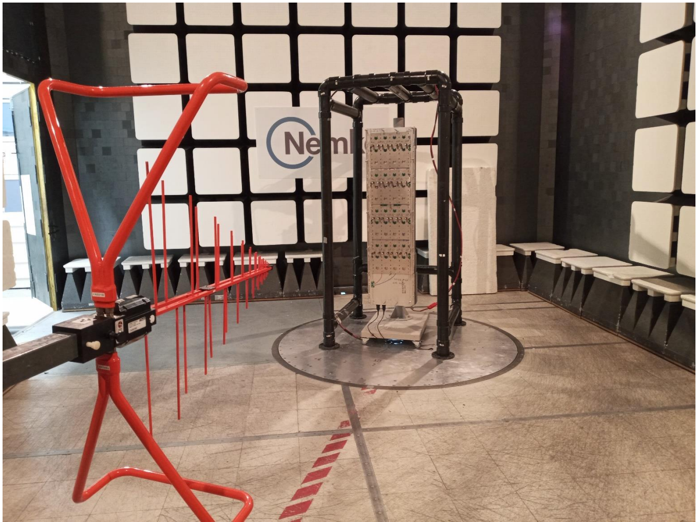
Figure 3.5-2: EUT Set-up for Radiated Compliance Testing
