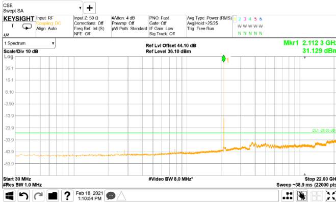
Figure 8.2-1: Conducted spurious emissions of 5 MHz low channel, single carrier operation
