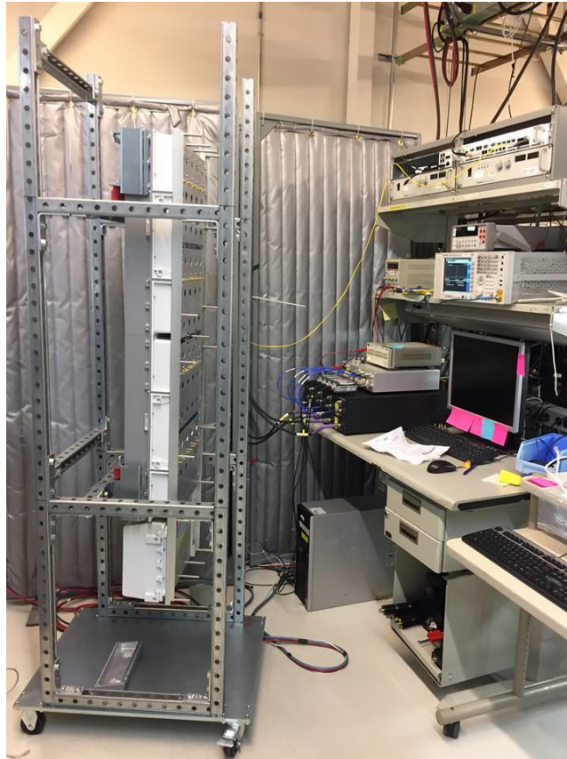
Figure 3.6-1: Test / Measurement Equipment - Set up for Radio Compliance Testing
