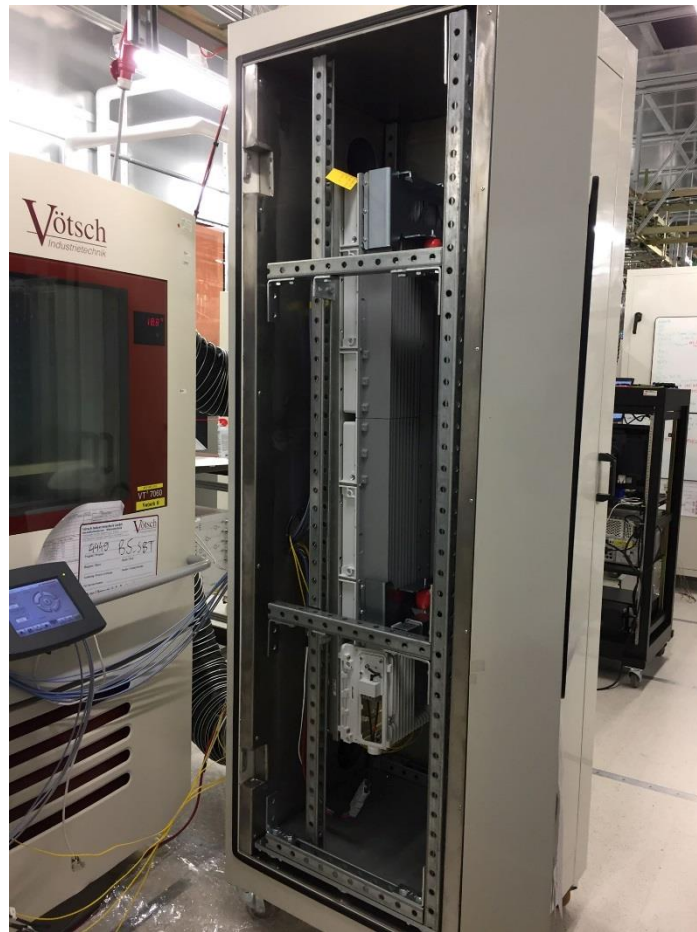
Figure 3.6-2: EUT Set-up for Radio Compliance Testing
