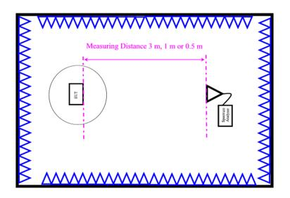
30 MHz - 60 GHz the measuring distance was 3m60 - 150 GHz the measuring distance was 1.0m: 150 - 200 GHz the measuring distance was 0.5m
