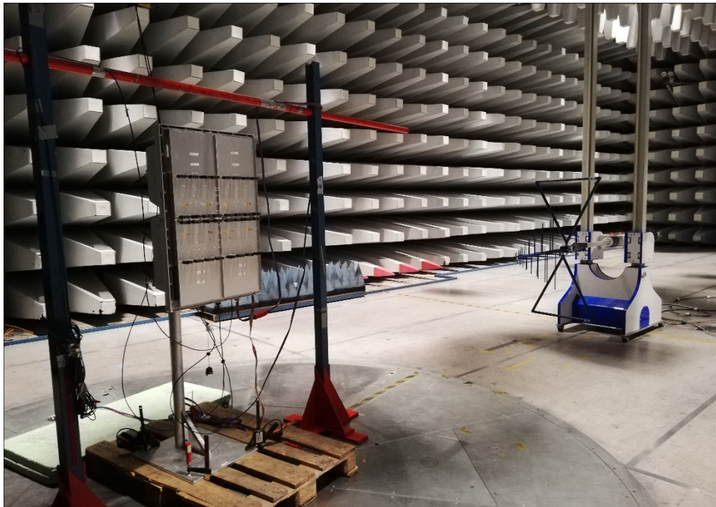
Figure 19 - Test Setup - 30 MHz to 1 GHz
