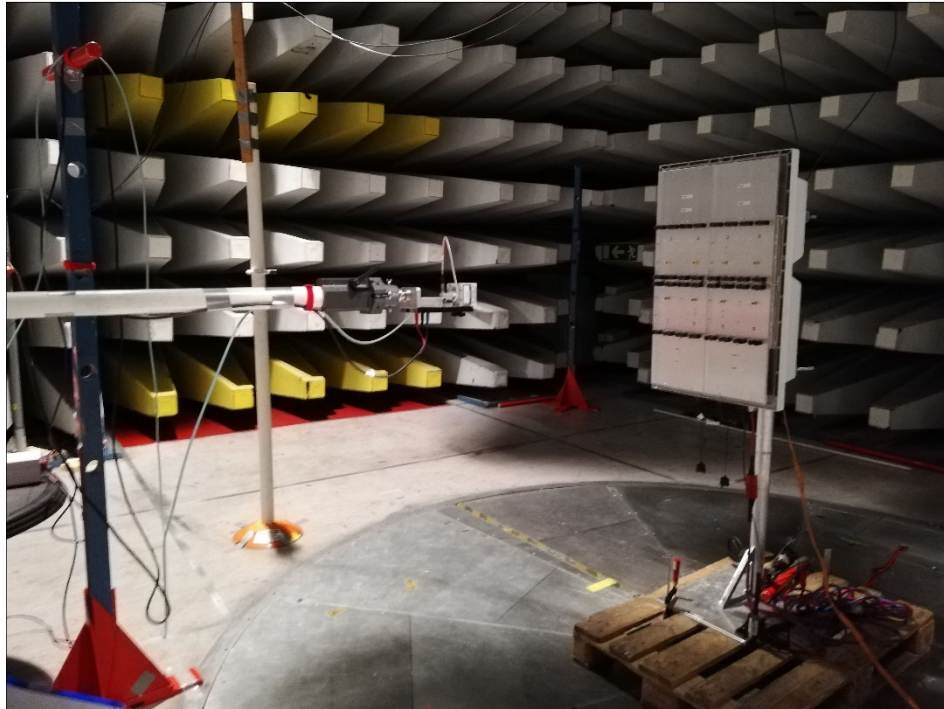
Figure 21 - Test Setup - 18 GHz to 40 GHz
