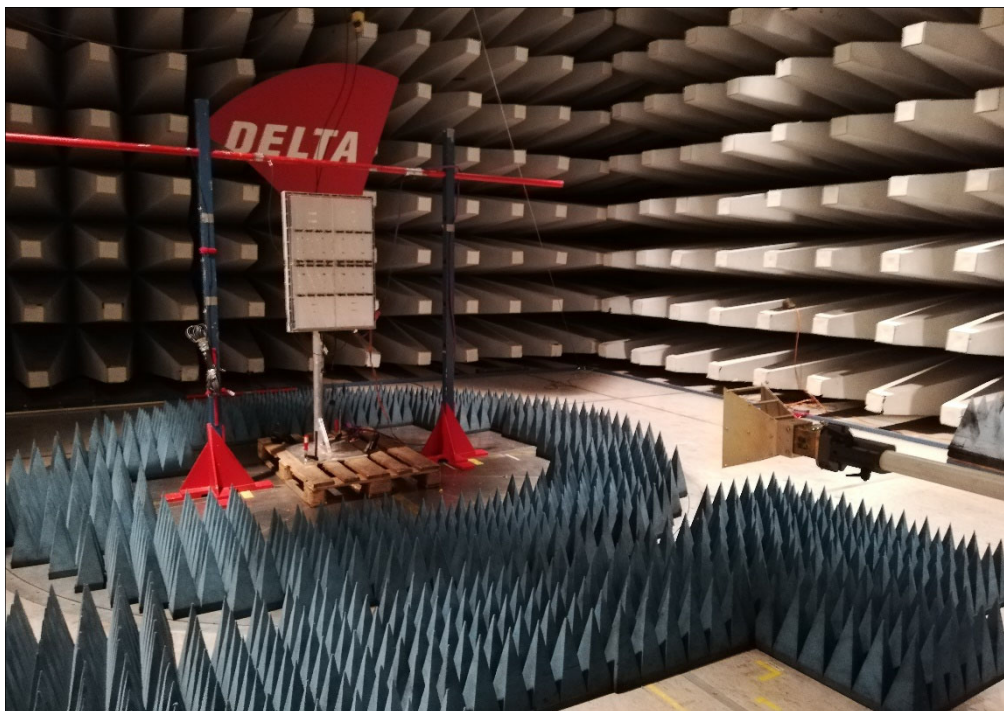
Figure 20 - Test Setup - 1 GHz to 18 GHz
