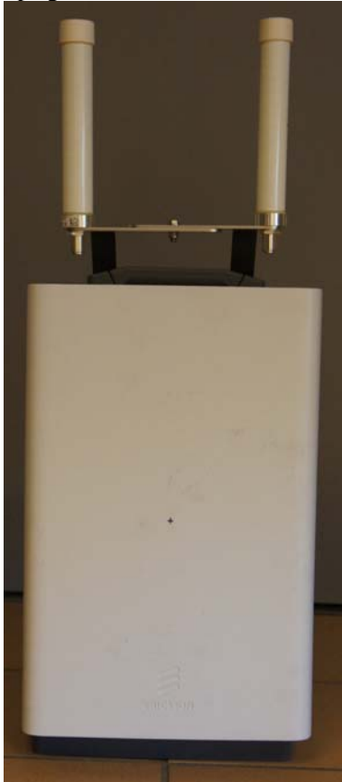
Front side with Semi-integrated omni antenna, upright mounted
