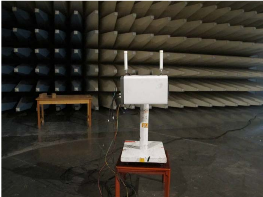
Semi-integrated Omni antenna KRE 101 2233/1, side mounted Maximum PEAK Output Power – Radiated (EIRP)
