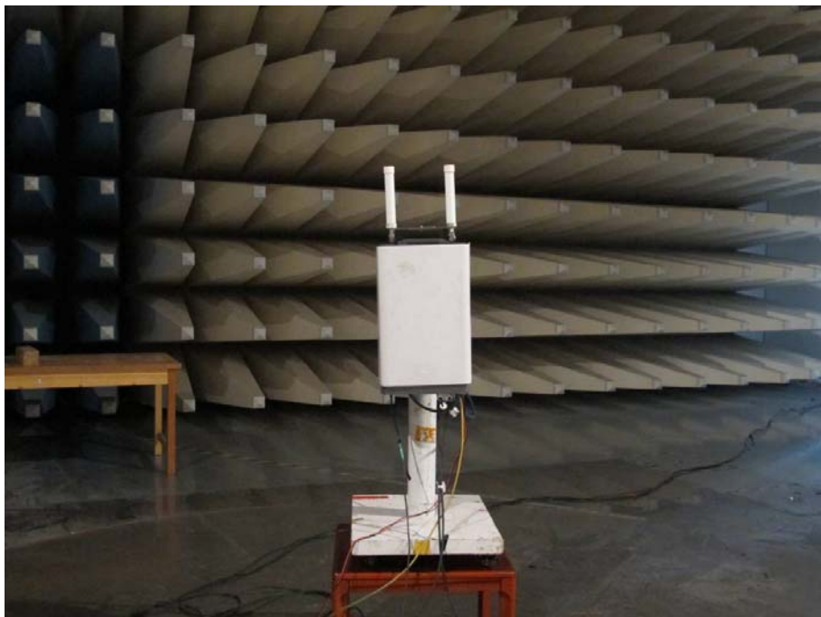
Semi-integrated Omni antenna KRE 101 2233/1, upright mounted Maximum PEAK Output Power – Radiated (EIRP)
