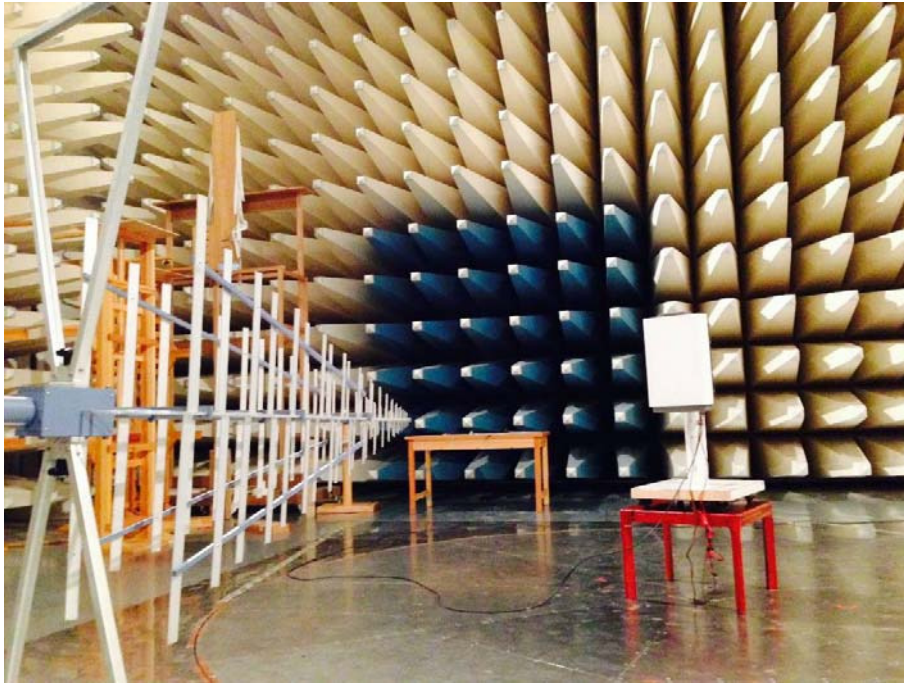
Integrated antenna KRE 101 2134/1, upright mounted
