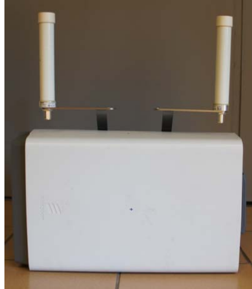
Front side with Semi-integrated omni antenna, side mounted
