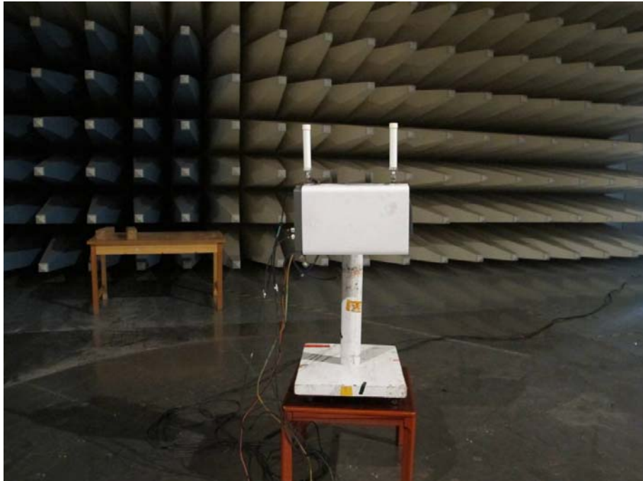
Maximum PEAK Output Power – Radiated (EIRP) Semi-integrated Omni antenna KRE 101 2233/1, side mounted
