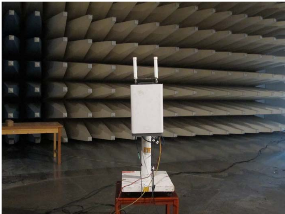
Maximum PEAK Output Power – Radiated (EIRP) Semi-integrated Omni antenna KRE 101 2233/1, upright mounted
