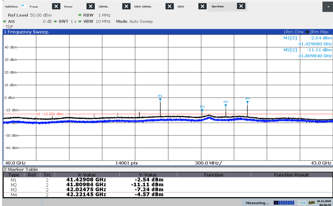
Diagram 30: 40 – 43 GHz, Modulation QPSK, Symbolic name: WC6Lo 100 , EIRP Vertical polarization
