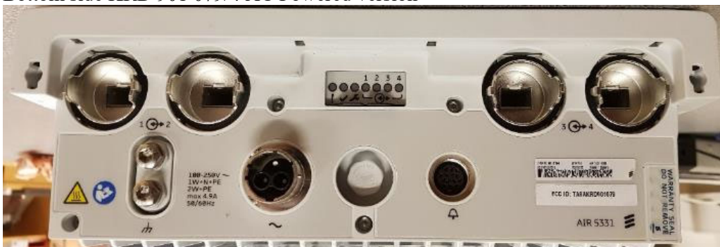
Bottom side KRD 901 079/4 AC Powered version
