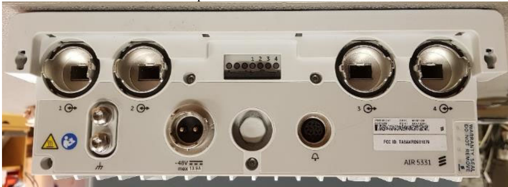
Bottom side KRD 901 079/4 AC Powered version
