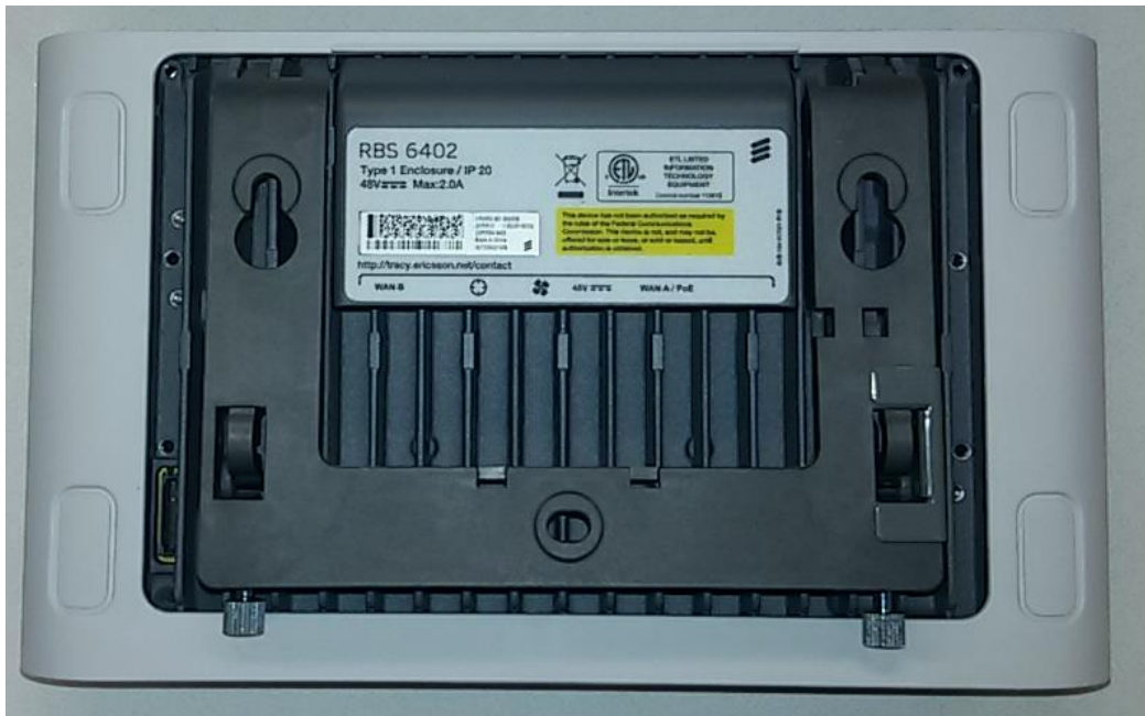
Figure 2 Back side with wall mount and locking plate attached
