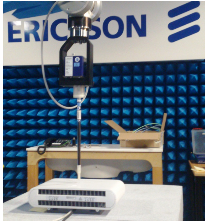
Figure C.1 EUT positioned for field strength measurements in the front position using the DASY5 near-field scanner.
