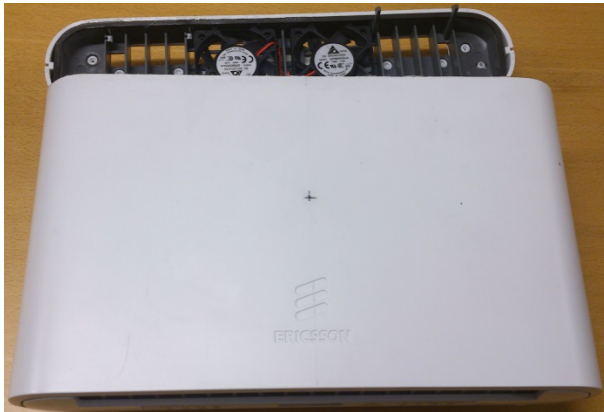
Figure A.2 EUT with the fan module opened
