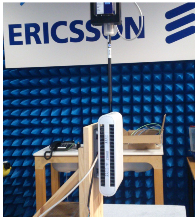
Figure C.2 EUT positioned for field strength measurements in the right side using the DASY5 near-field scanner.
