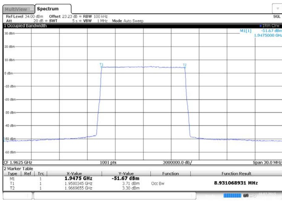
Antenna A - Modulation 64QAM - Carrier Bandwidth 15.0 MHz - Channel Position M - Measurement 99 % BW
