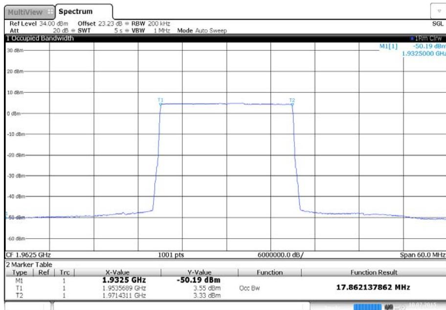
Antenna A - Modulation QPSK - Carrier Bandwidth 20.0 MHz - Channel Position T - Measurement 99 % BW
