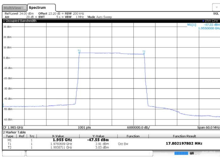
Antenna A - Modulation QPSK - Carrier Bandwidth 5.0 MHz - Channel Position B - Measurement -26 dB BW
