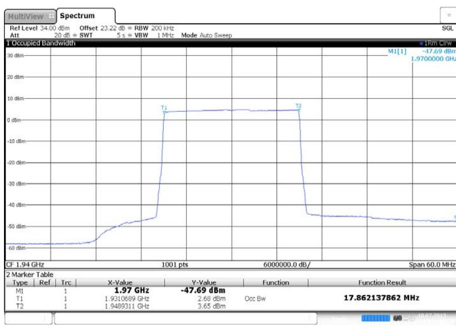
Antenna A - Modulation QPSK - Carrier Bandwidth 20.0 MHz - Channel Position M - Measurement 99 % BW
