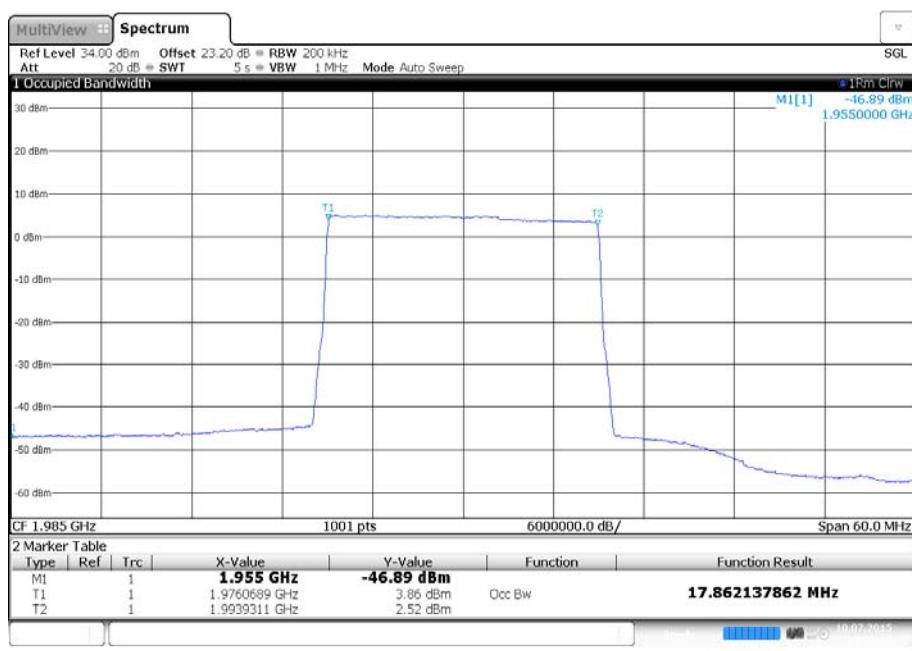
Antenna A - Modulation 64QAM - Carrier Bandwidth 5.0 MHz - Channel Position B - Measurement -26 dB BW
