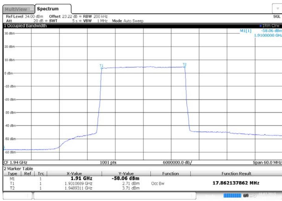
Antenna A - Modulation 64QAM - Carrier Bandwidth 20.0 MHz - Channel Position M - Measurement 99 % BW
