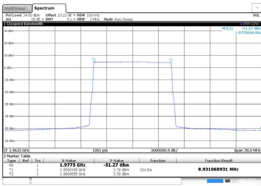
Antenna A - Modulation QPSK - Carrier Bandwidth 15.0 MHz - Channel Position M - Measurement 99 % BW
