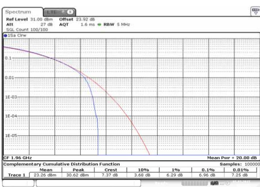
Modulation 16QAM - Bandwidth 10.0 MHz - Antenna A - Channel Position M
