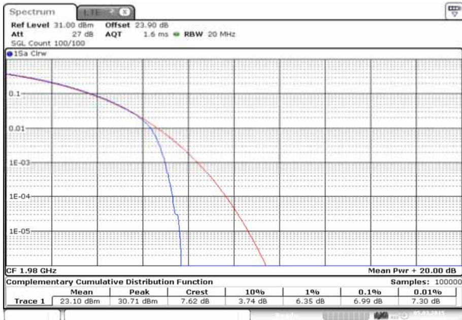
Modulation QPSK - Bandwidth 20.0 MHz - Antenna D - Channel Position T
