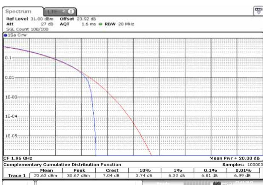
Modulation 16QAM - Bandwidth 15.0 MHz - Antenna C - Channel Position M
