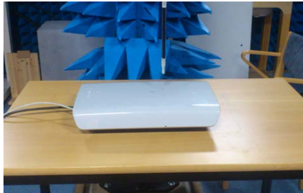
Figure C.1 EUT positioned for field strength measurements in the front position using the DASYS5 near-field scanner.
