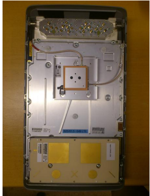
Figure A.1 Front view of the EUT and EUT with radome removed showing the LTE and Wi-Fi antennas.
