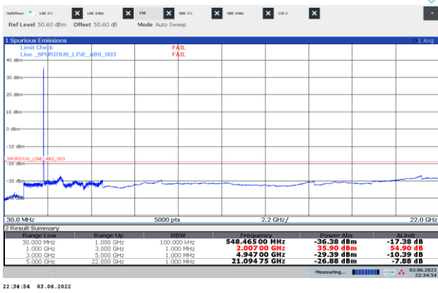
Figure 8.7-23: Conducted spurious emissions of NR15 MHz mid channel, single carrier operation
