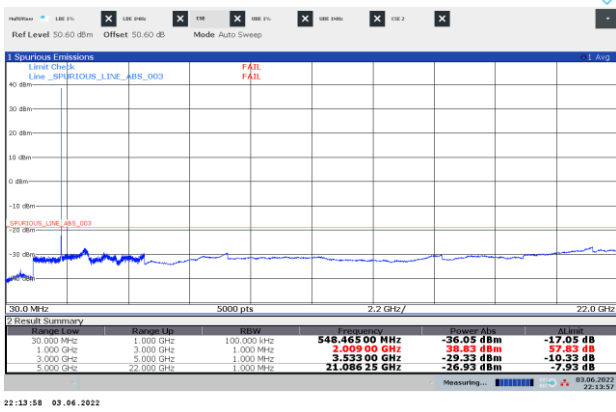
Figure 8.7-5: Conducted spurious emissions of LTE 5 MHz mid channel with IB-IoT2, single carrier operation
