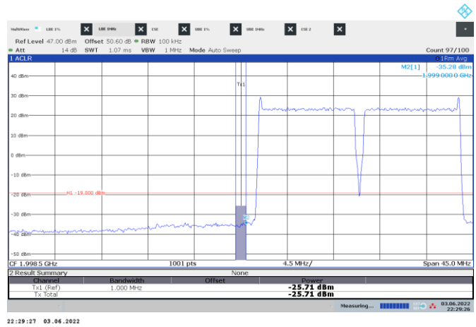
Figure 8.7-57: Conducted emission 1 MHz away from the lower band edge
