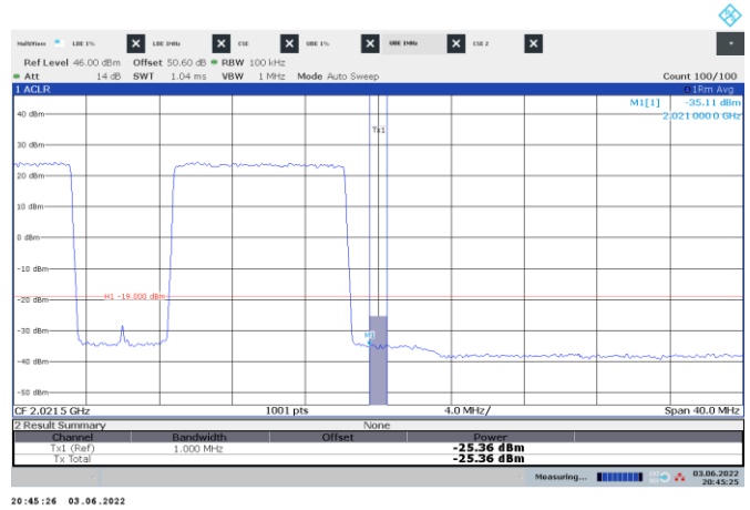
Figure 8.7-83: Conducted emission 1 MHz away from the upper band edge
