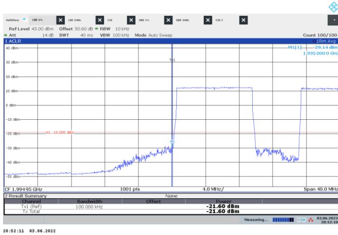
Figure 8.6-121: Conducted emission at the lower band edge
