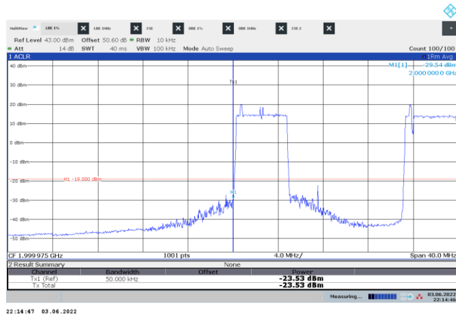
Figure 8.7-52: Conducted emission at the lower band edge
