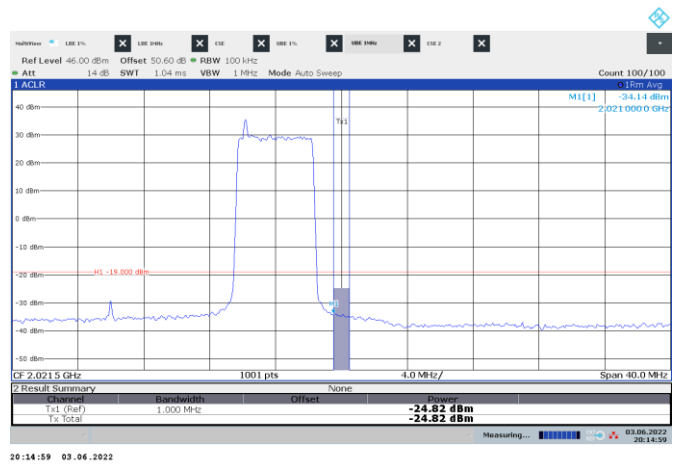
Figure 8.7-35: Conducted emission 1 MHz away from the upper band edge
