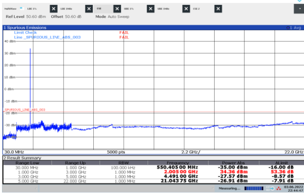
Figure 8.7-25: Conducted spurious emissions of NR20 MHz mid channel, single carrier operation
