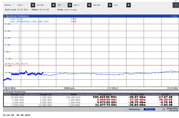
Figure 8.7-2: Conducted spurious emissions of LTE 5 MHz mid channel with IB-IoT1, single carrier operation
