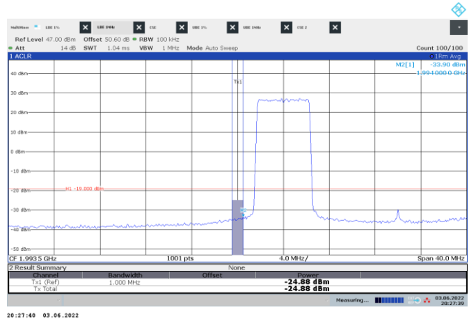
Figure 8.6-110: Conducted emission 1 MHz away from the lower band edge
