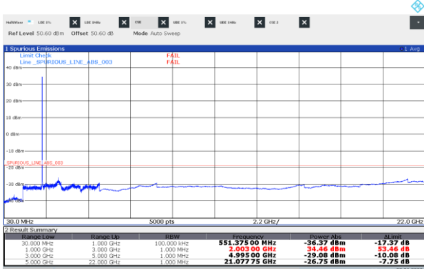
Figure 8.7-25: Conducted spurious emissions of NR20 MHz mid channel, single carrier operation
