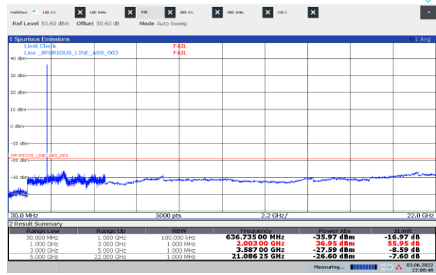
Figure 8.7-26: Conducted spurious emissions of NR 5 MHz, two-carrier operation
