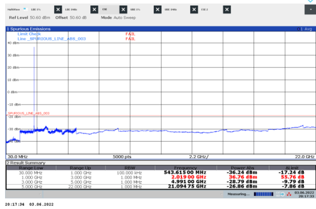
Figure 8.7-6: Conducted spurious emissions of LTE 5 MHz top channel with IB-IoT2, single carrier operation
