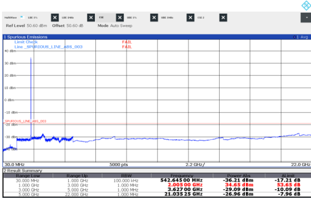
Figure 8.7-9: Conducted spurious emissions of LTE 10 MHz top channel, single carrier operation
