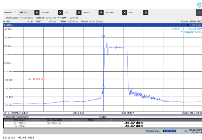
Figure 8.7-36: Conducted emission at the lower band edge
