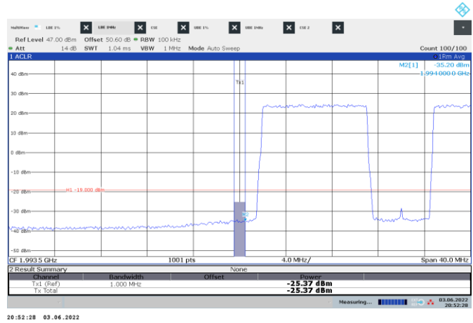
Figure 8.6-122: Conducted emission 1 MHz away from the lower band edge
