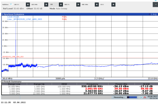
Figure 8.7-1: Conducted spurious emissions of LTE 5 MHz low channel with IB-IoT1, single carrier operation
