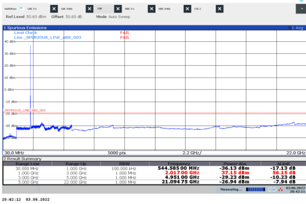
Figure 8.7-21: Conducted spurious emissions of NR10 MHz top channel, single carrier operation
