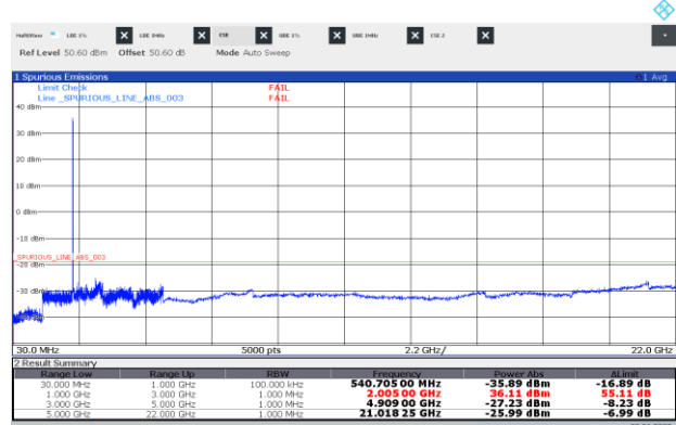
Figure 8.7-26: Conducted spurious emissions of NR 5 MHz, two-carrier operation
