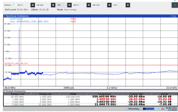
Figure 8.7-8: Conducted spurious emissions of LTE 10 MHz mid channel, single carrier operation
