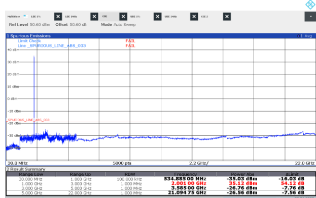
Figure 8.7-8: Conducted spurious emissions of LTE 10 MHz mid channel, single carrier operation
