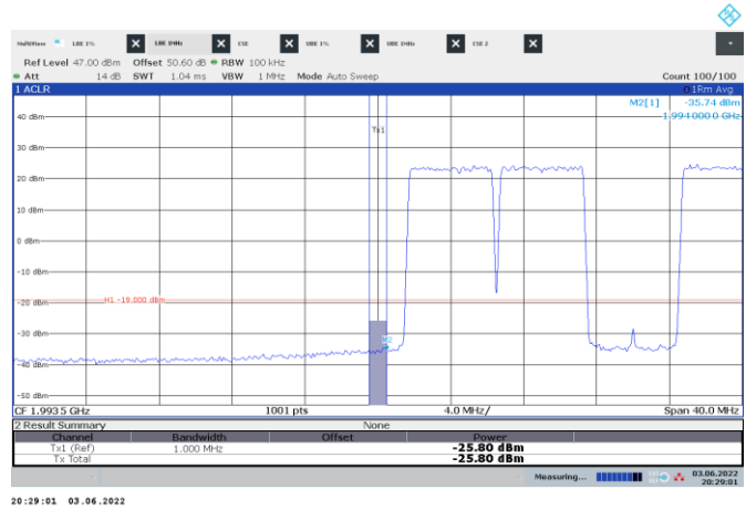
Figure 8.6-114: Conducted emission 1 MHz away from the lower band edge
