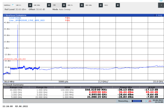
Figure 8.7-20: Conducted spurious emissions of NR10 MHz mid channel, single carrier operation
