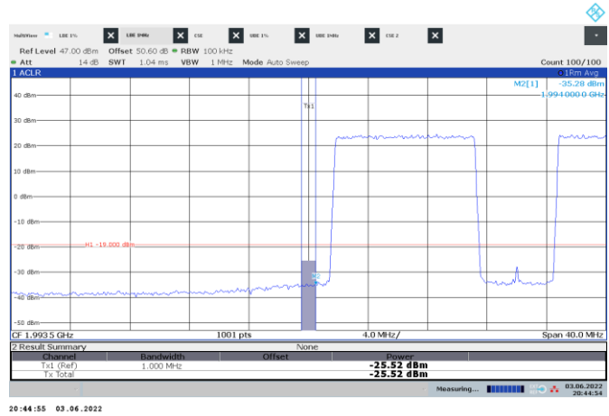
Figure 8.6-106: Conducted emission 1 MHz away from the lower band edge
