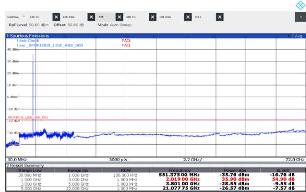
Figure 8.6-10: Conducted spurious emissions of LTE 15 MHz low channel, single carrier operation
