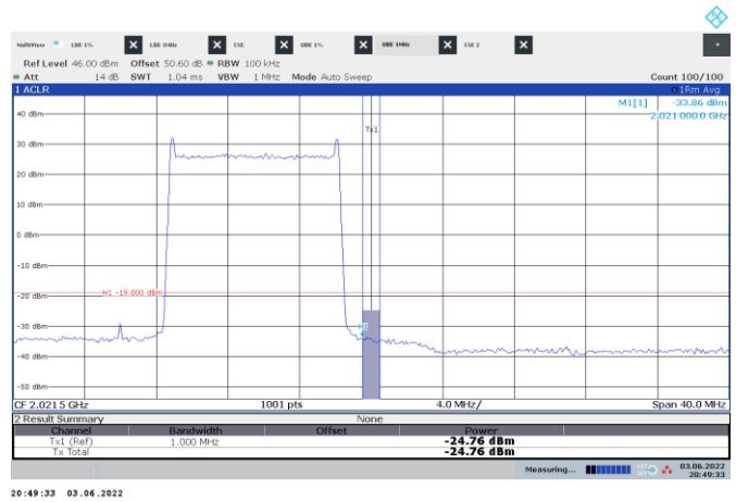
Figure 8.6-52: Conducted emission 1 MHz away from the upper band edge
