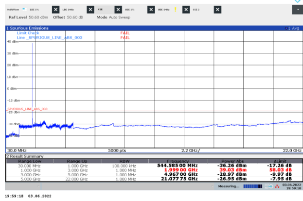
Figure 8.6-20: Conducted spurious emissions of NR5 MHz low channel, single carrier operation
