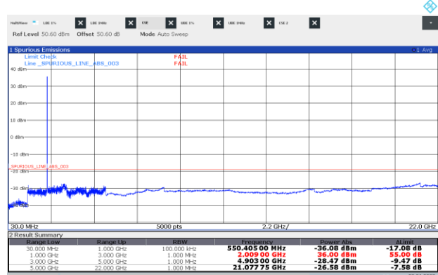
Figure 8.6-8: Conducted spurious emissions of LTE 10 MHz mid channel, single carrier operation
