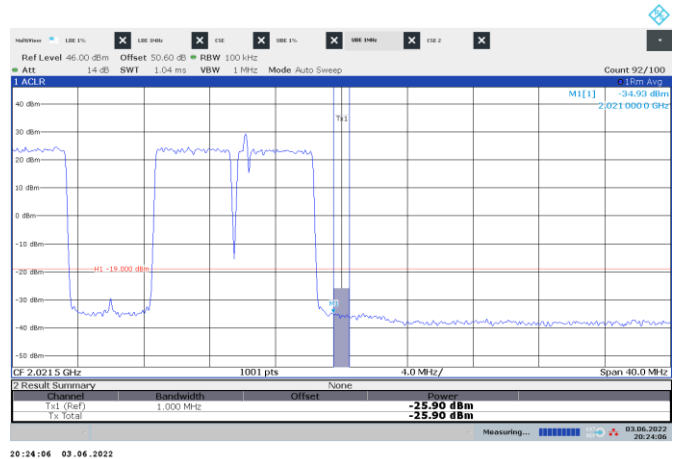
Figure 8.6-68: Conducted emission 1 MHz away from the upper band edge
