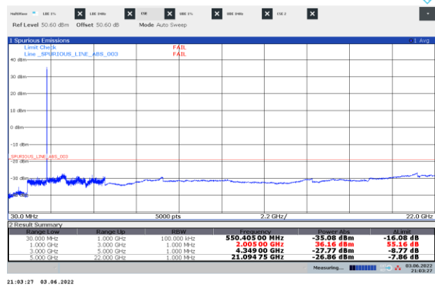
Figure 8.6-26: Conducted spurious emissions of NR15 MHz low channel, single carrier operation
