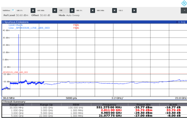
Figure 8.6-9: Conducted spurious emissions of LTE 10 MHz top channel, single carrier operation
