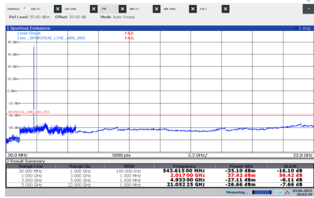
Figure 8.6-32: Conducted spurious emissions of NR 5 MHz, two-carrier operation
