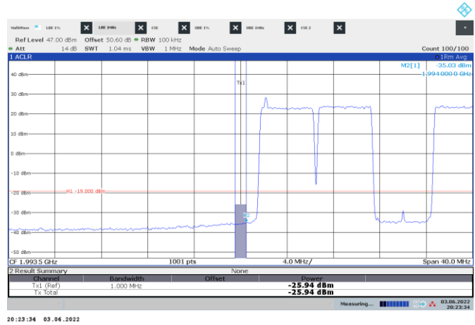
Figure 8.6-66: Conducted emission 1 MHz away from the lower band edge
