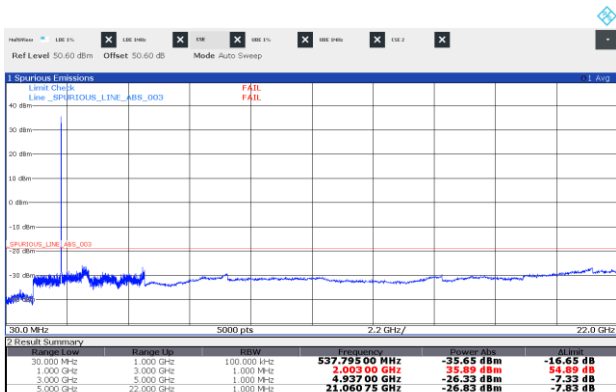
Figure 8.6-33: Conducted spurious emissions of NR 5 MHz, three-carrier operation
