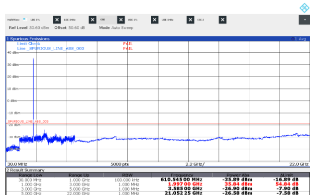
Figure 8.6-34: Conducted spurious emissions of NR 5 MHz, four-carrier operation
