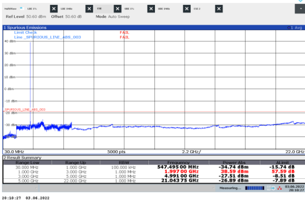
Figure 8.6-1: Conducted spurious emissions of LTE 5 MHz low channel with IB-IoT1, single carrier operation
