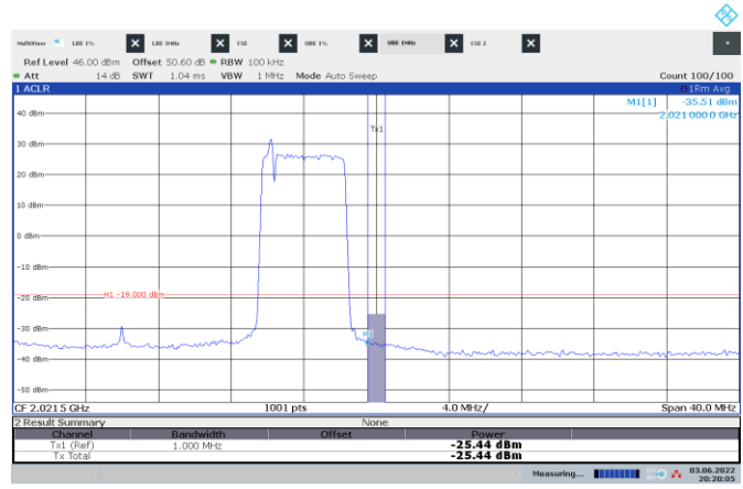
Figure 8.6-64: Conducted emission 1 MHz away from the upper band edge
