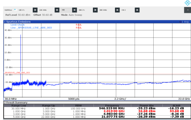
Figure 8.6-32: Conducted spurious emissions of NR 5 MHz, two-carrier operation
