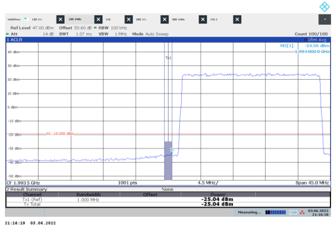
Figure 8.6-90: Conducted emission 1 MHz away from the lower band edge
