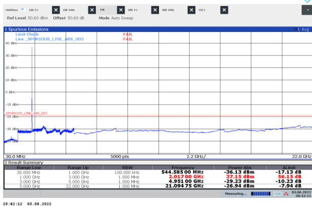
Figure 8.6-25: Conducted spurious emissions of NR10 MHz top channel, single carrier operation
