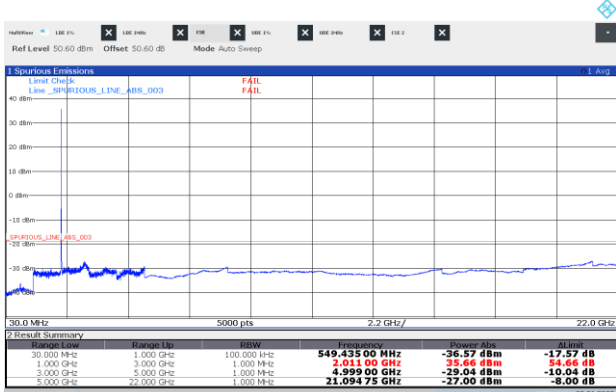
Figure 8.6-7: Conducted spurious emissions of LTE 10 MHz low channel, single carrier operation
