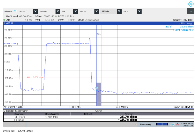
Figure 8.6-76: Conducted emission 1 MHz away from the upper band edge
