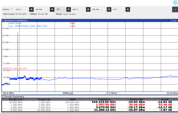
Figure 8.6-31: Conducted spurious emissions of NR20 MHz top channel, single carrier operation
