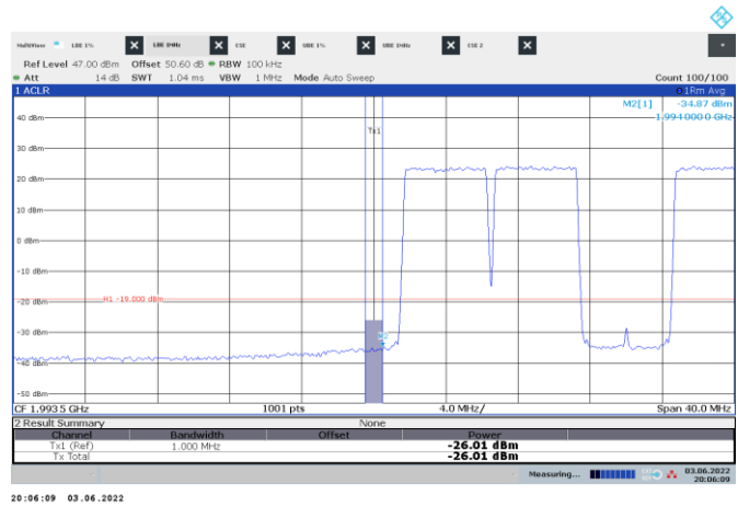
Figure 8.6-98: Conducted emission 1 MHz away from the lower band edge
