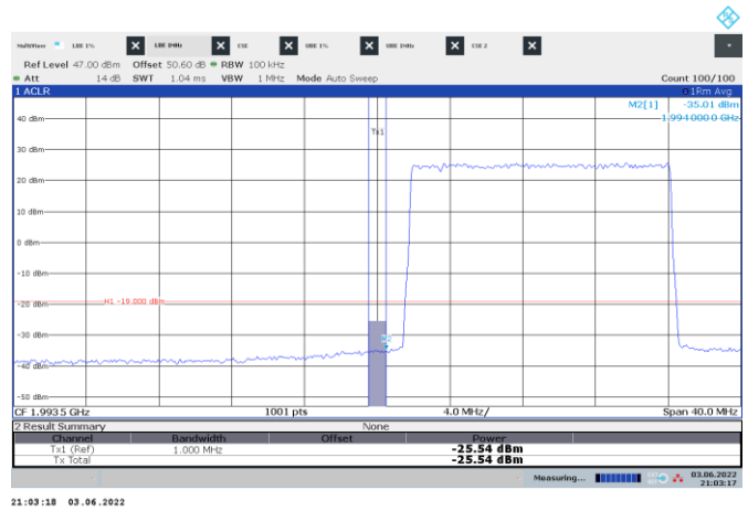
Figure 8.6-86: Conducted emission 1 MHz away from the lower band edge
