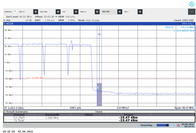
Figure 8.6-72: Conducted emission 1 MHz away from the upper band edge
