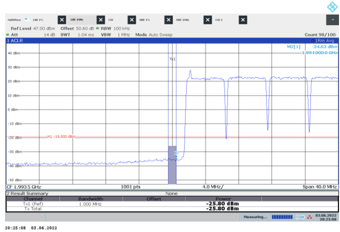
Figure 8.6-70: Conducted emission 1 MHz away from the lower band edge
