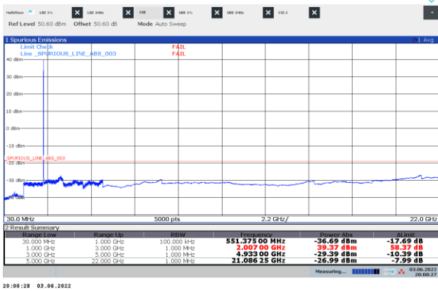
Figure 8.6-21: Conducted spurious emissions of NR5 MHz mid channel, single carrier operation
