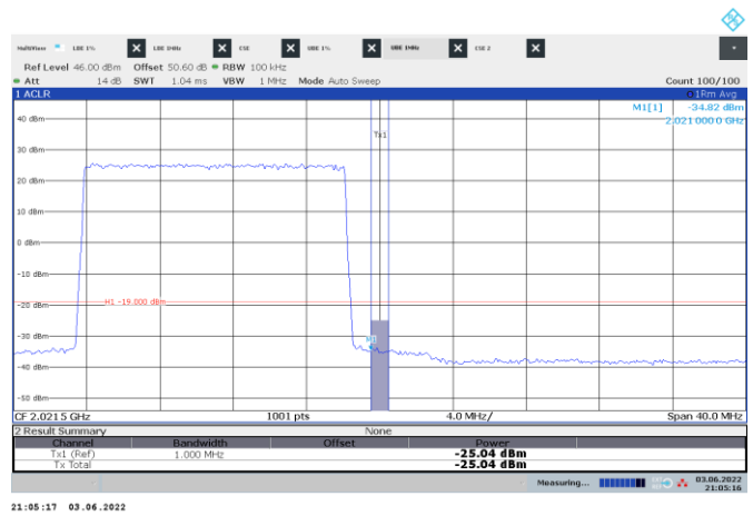
Figure 8.6-88: Conducted emission 1 MHz away from the upper band edge
