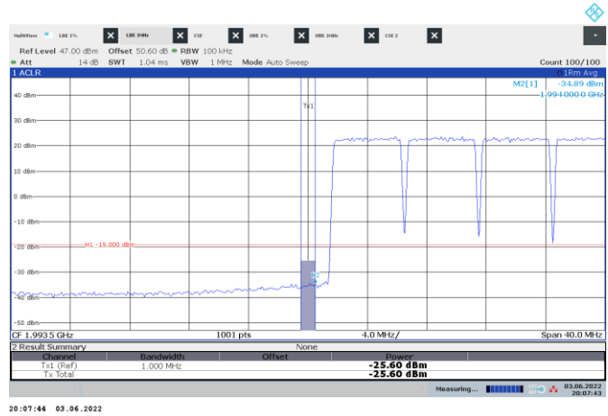
Figure 8.6-102: Conducted emission 1 MHz away from the lower band edge
