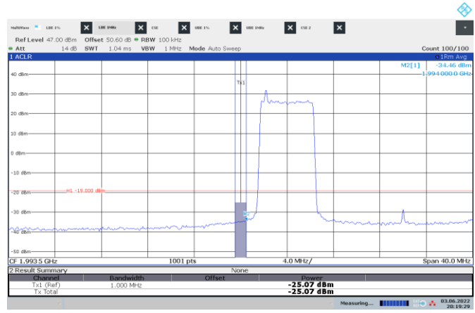
Figure 8.6-62: Conducted emission 1 MHz away from the lower band edge
