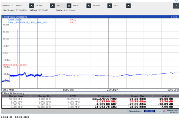
Figure 8.6-19: Conducted spurious emissions of LTE 10 MHz, two-carrier operation
