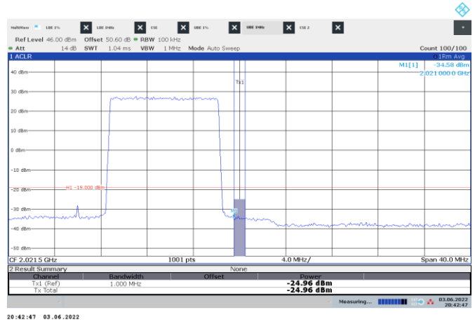
Figure 8.6-84: Conducted emission 1 MHz away from the upper band edge
