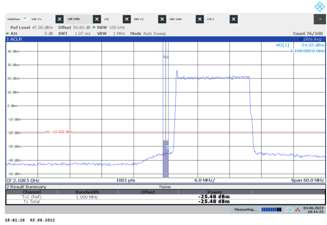
Figure 8.4-80: Conducted emission 1 MHz away from the lower band edge
