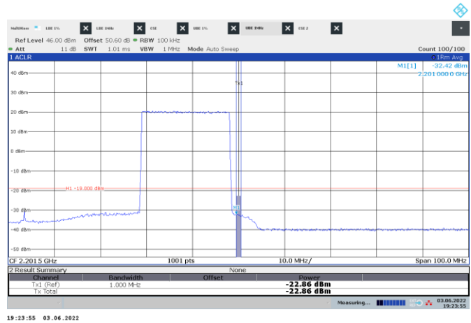
Figure 8.4-150: Conducted emission 1 MHz away from the upper band edge
