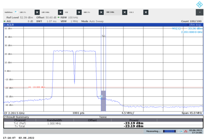
Figure 8.4-158: Conducted emission 1 MHz away from the upper band edge
