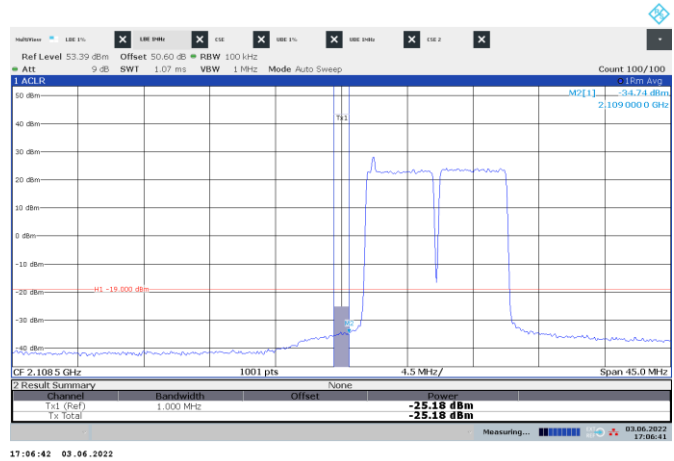
Figure 8.4-72: Conducted emission 1 MHz away from the lower band edge
