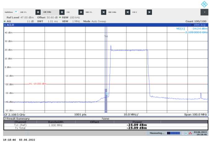
Figure 8.4-92: Conducted emission 1 MHz away from the lower band edge
