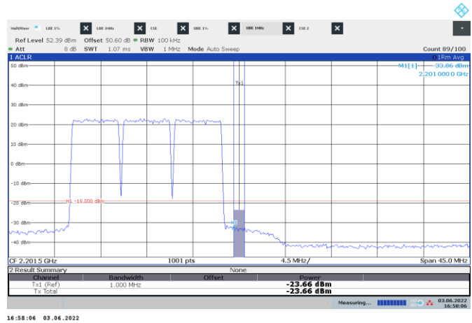
Figure 8.4-126: Conducted emission 1 MHz away from the upper band edge
