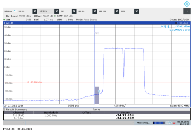
Figure 8.4-156: Conducted emission 1 MHz away from the lower band edge
