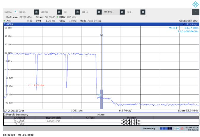
Figure 8.4-170: Conducted emission 1 MHz away from the upper band edge
