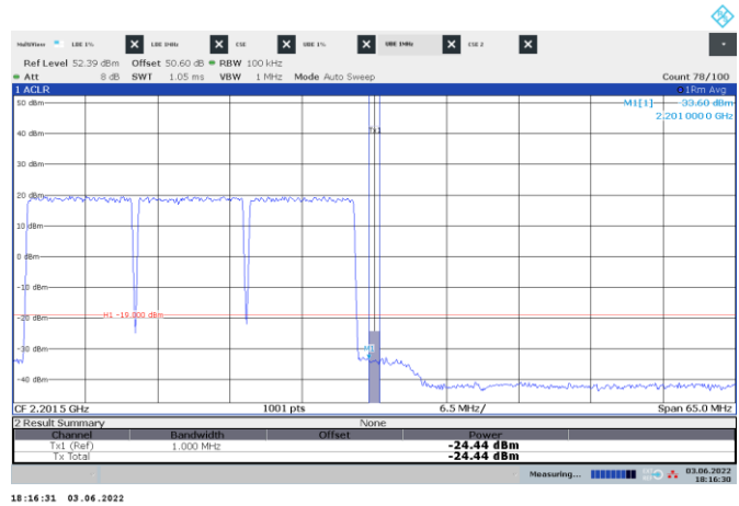
Figure 8.4-134: Conducted emission 1 MHz away from the upper band edge
