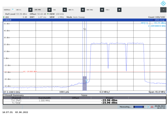
Figure 8.4-124: Conducted emission 1 MHz away from the lower band edge
