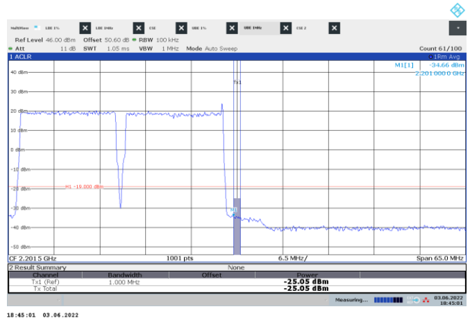
Figure 8.4-86: Conducted emission 1 MHz away from the upper band edge
