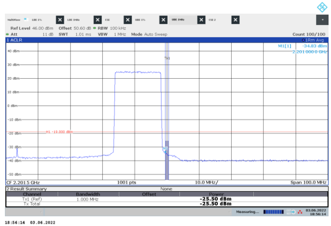
Figure 8.4-110: Conducted emission 1 MHz away from the upper band edge
