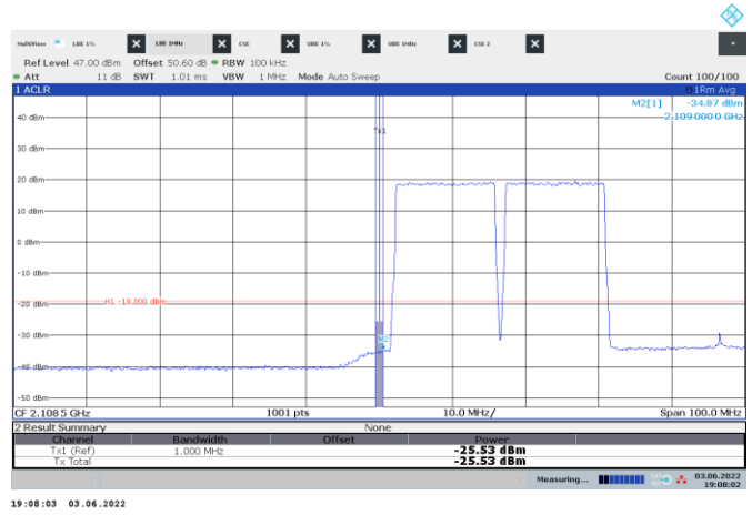
Figure 8.4-172: Conducted emission 1 MHz away from the lower band edge
