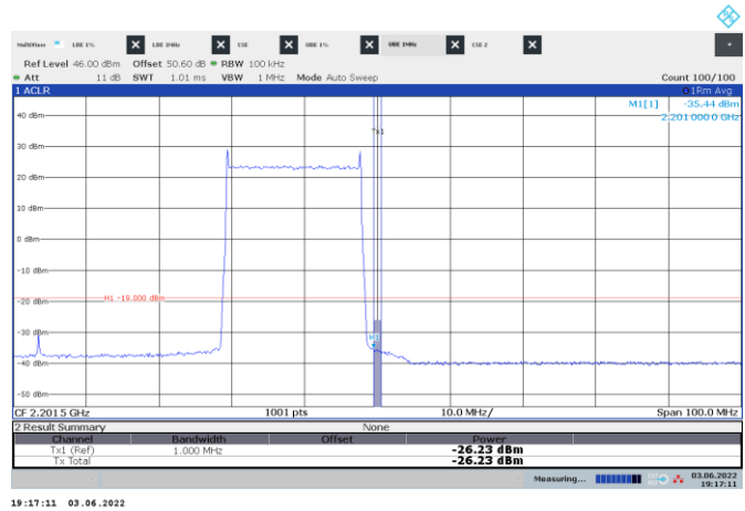
Figure 8.4-66: Conducted emission 1 MHz away from the upper band edge
