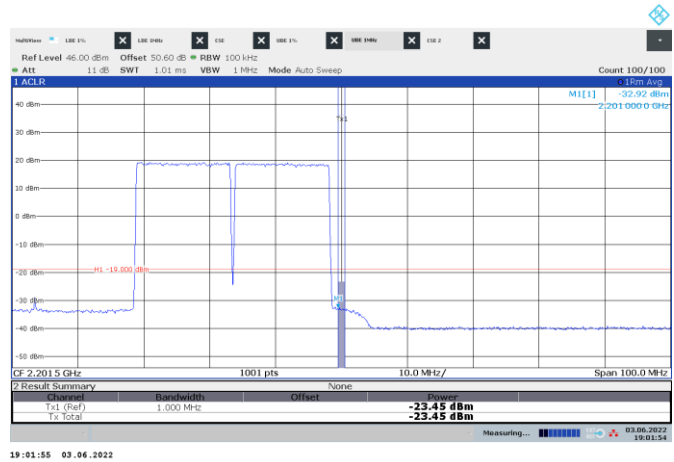
Figure 8.4-142: Conducted emission 1 MHz away from the upper band edge
