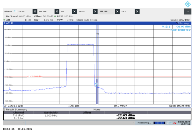
Figure 8.4-138: Conducted emission 1 MHz away from the upper band edge
