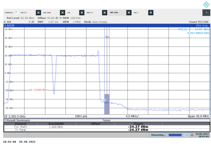
Figure 8.4-166: Conducted emission 1 MHz away from the upper band edge
