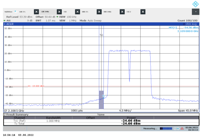
Figure 8.4-120: Conducted emission 1 MHz away from the lower band edge
