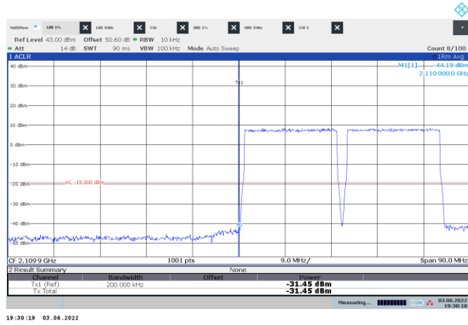
Figure 8.4-179: Conducted emission at the lower band edge
