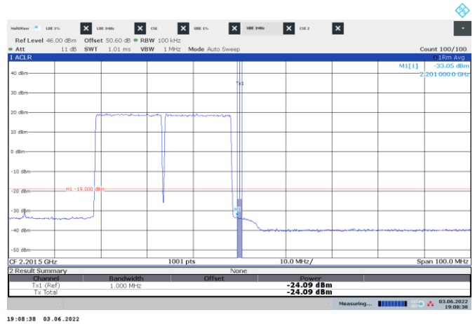
Figure 8.4-174: Conducted emission 1 MHz away from the upper band edge
