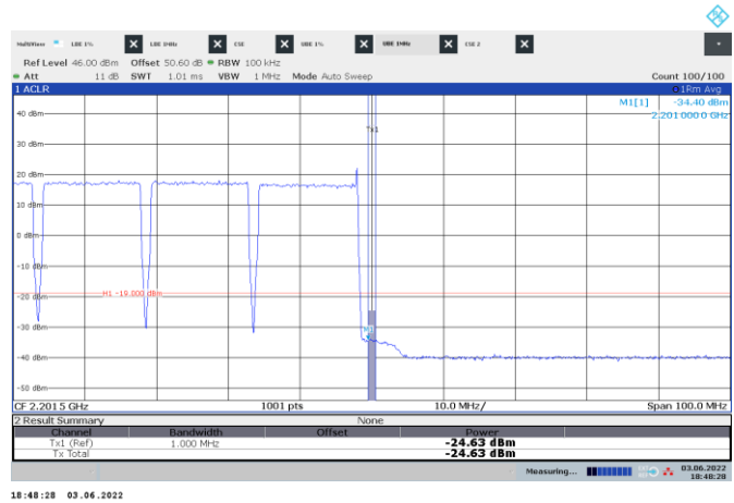
Figure 8.4-90: Conducted emission 1 MHz away from the upper band edge
