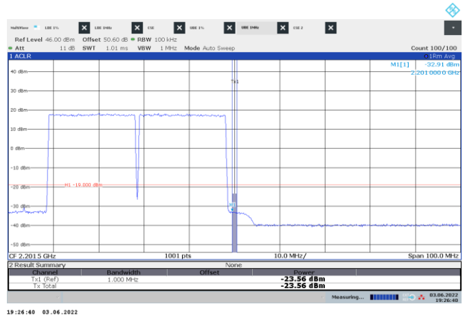
Figure 8.4-154: Conducted emission 1 MHz away from the upper band edge
