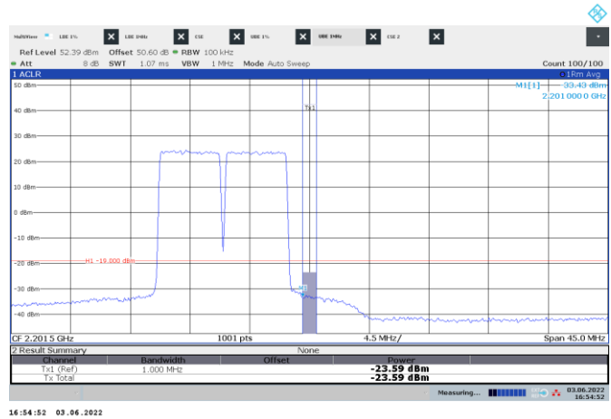
Figure 8.4-122: Conducted emission 1 MHz away from the upper band edge
