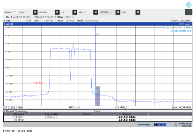
Figure 8.4-74: Conducted emission 1 MHz away from the upper band edge
