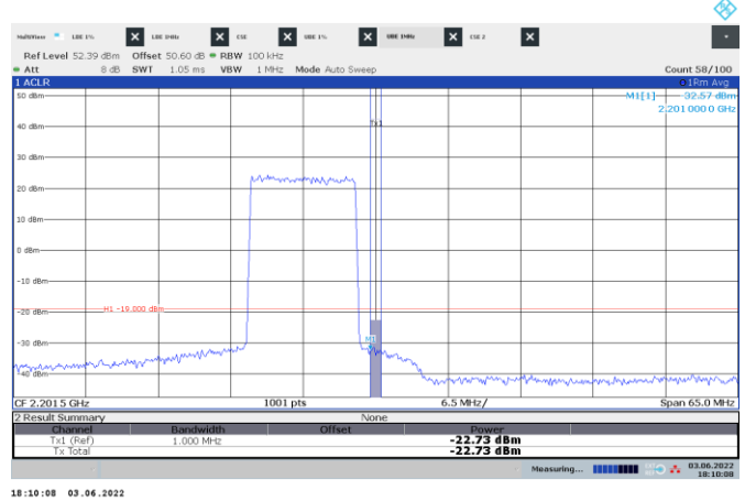
Figure 8.4-130: Conducted emission 1 MHz away from the upper band edge
