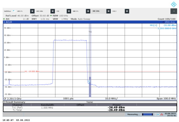
Figure 8.4-114: Conducted emission 1 MHz away from the upper band edge
