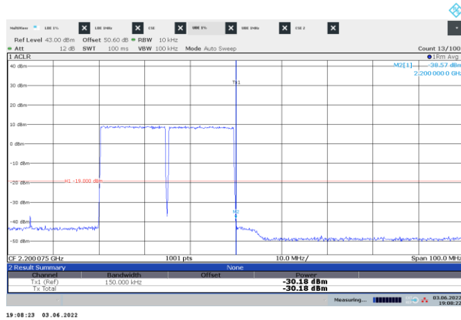
Figure 8.4-173: Conducted emission at the upper band edge
