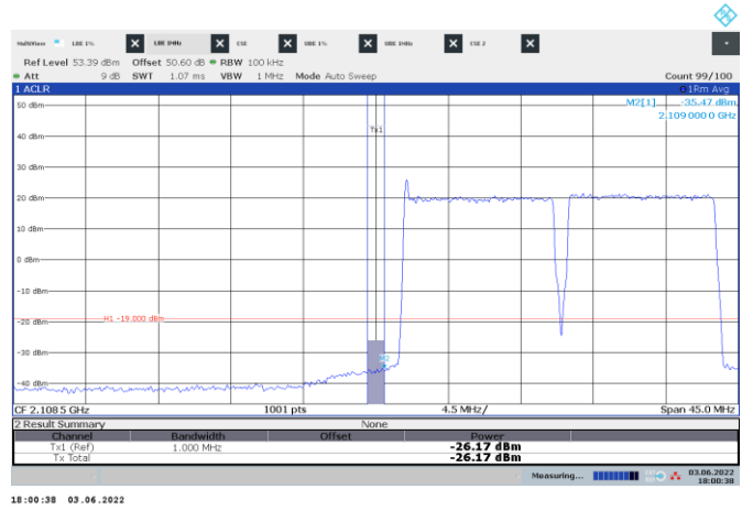
Figure 8.4-164: Conducted emission 1 MHz away from the lower band edge
