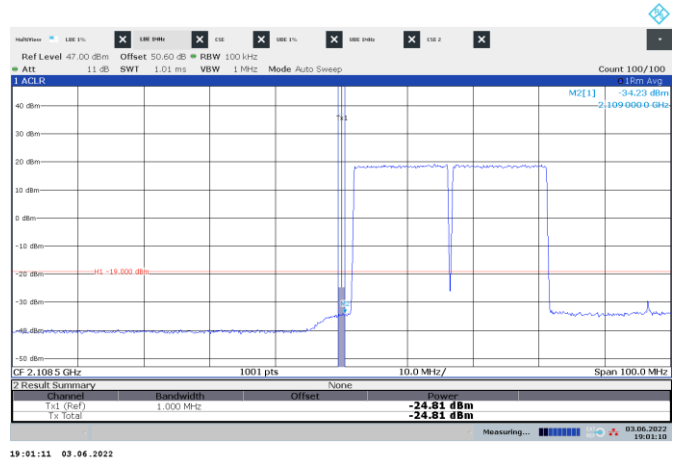
Figure 8.4-140: Conducted emission 1 MHz away from the lower band edge
