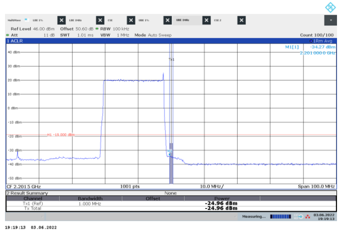
Figure 8.4-94: Conducted emission 1 MHz away from the upper band edge
