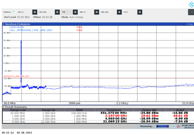
Figure 8.4-47: Conducted spurious emissions of multi-RAT operation, 3xLTE 10 MHz and 3xNR 10 MHz, six-carrier operation
