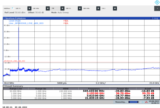
Figure 8.4-26: Conducted spurious emissions of NR10 MHz top channel, single carrier operation
