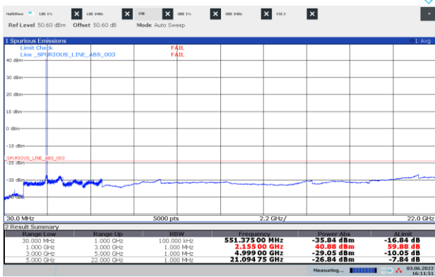
Figure 8.4-5: Conducted spurious emissions of LTE 5 MHz mid channel with IB-IoT2, single carrier operation
