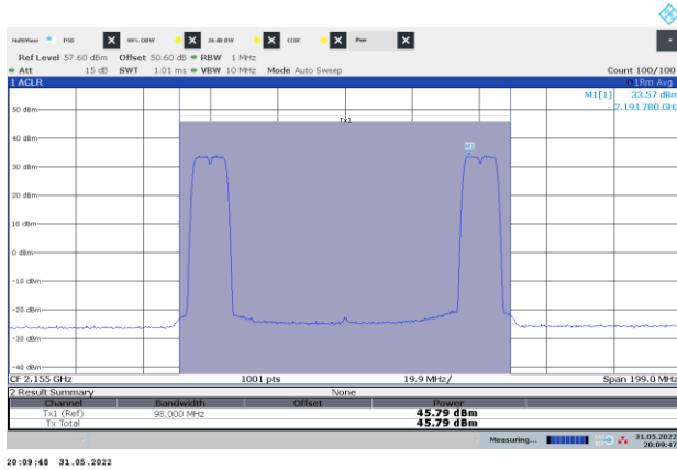
Figure 8.1-72: PSD and Output channel power of Multi-RAT, four carriers operation 2x LTE 5 MHz + 2x NR 5 MHz, sample plot
