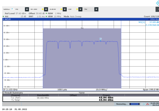
Figure 8.1-78: PSD and Output channel power of Multi-RAT, six carriers operation 3x LTE 15 MHz + 3x NR 15 MHz, sample plot
