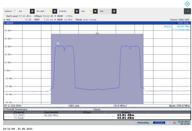
Figure 8.1-73: PSD and Output channel power of Multi-RAT, four carriers operation 2x LTE 10 MHz + 2x NR 10 MHz, sample plot
