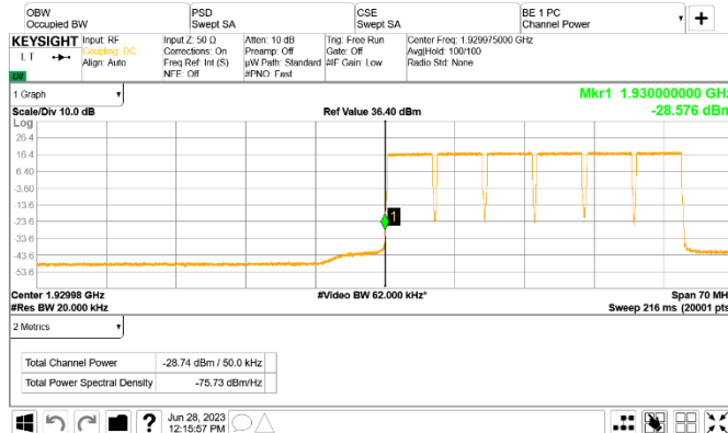
Figure 8.5-175: Conducted emission at the lower band edge
