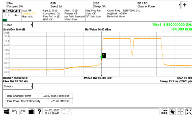
Figure 8.5-167: Conducted emission at the lower band edge
