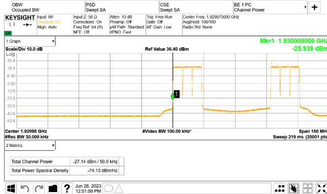
Figure 8.5-183: Conducted emission at the lower band edge
