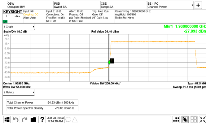
Figure 8.5-159: Conducted emission at the lower band edge
