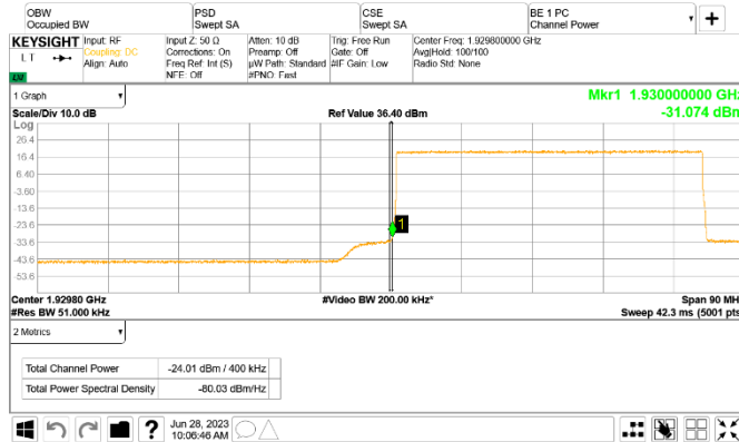
Figure 8.5-163: Conducted emission at the lower band edge
