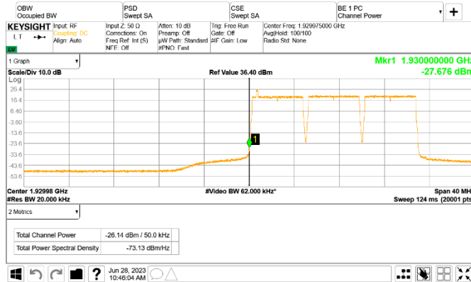
Figure 8.5-131: Conducted emission at the lower band edge
