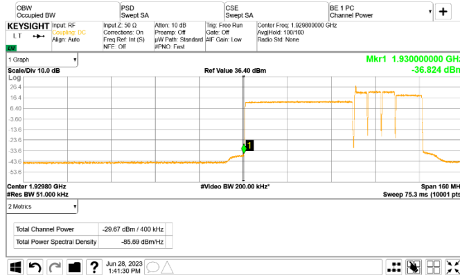
Figure 8.5-199: Conducted emission at the lower band edge
