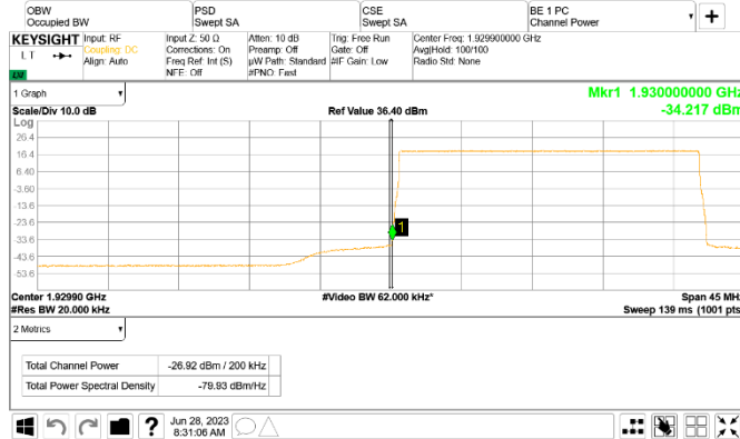
Figure 8.5-151: Conducted emission at the lower band edge
