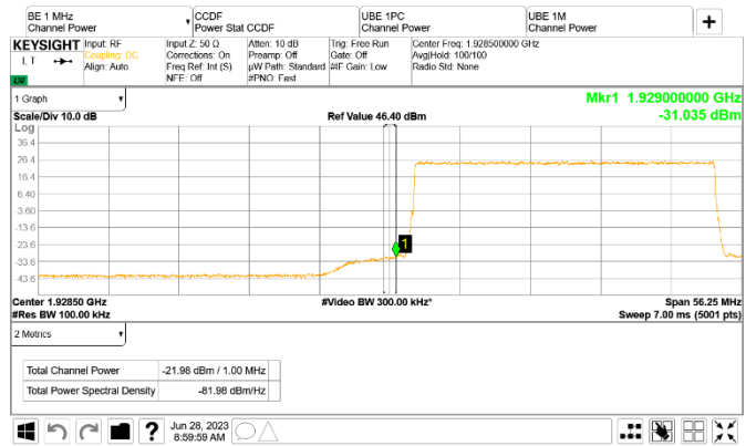
Figure 8.5-156: Conducted emission 1 MHz away from the lower band edge
