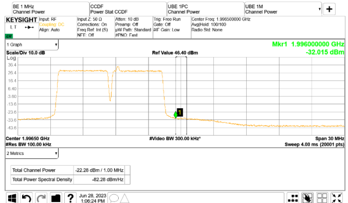
Figure 8.5-190: Conducted emission 1 MHz away from the upper band edge
