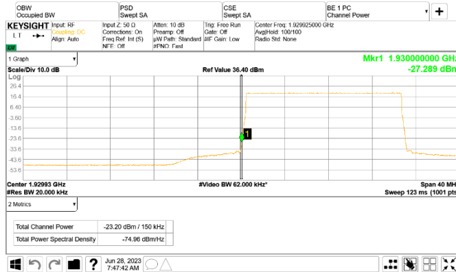
Figure 8.5-147: Conducted emission at the lower band edge
