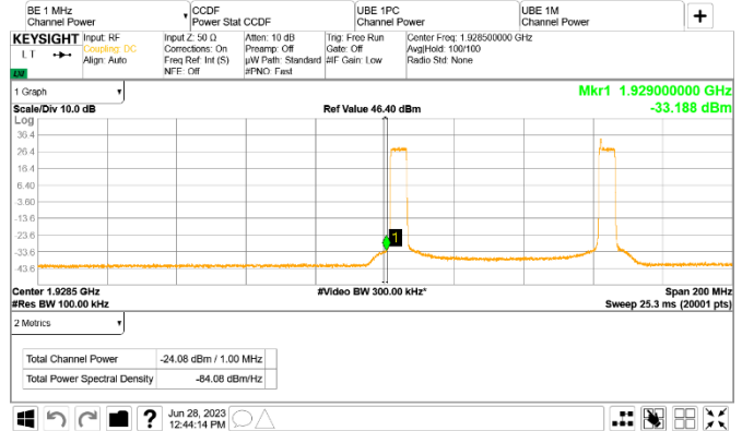
Figure 8.5-180: Conducted emission 1 MHz away from the lower band edge
