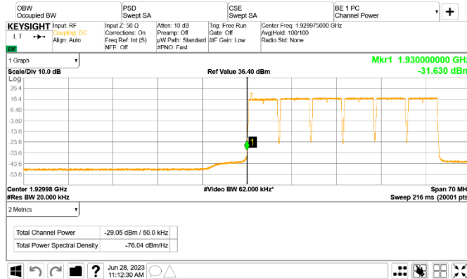
Figure 8.5-135: Conducted emission at the lower band edge
