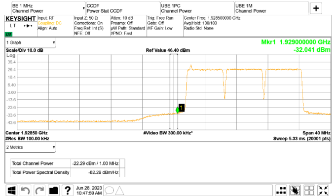
Figure 8.5-132: Conducted emission 1 MHz away from the lower band edge
