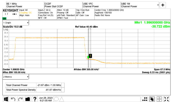
Figure 8.5-162: Conducted emission 1 MHz away from the upper band edge
