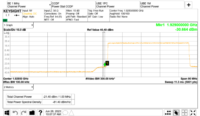
Figure 8.5-164: Conducted emission 1 MHz away from the lower band edge
