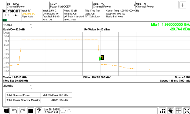
Figure 8.5-153: Conducted emission at the upper band edge
