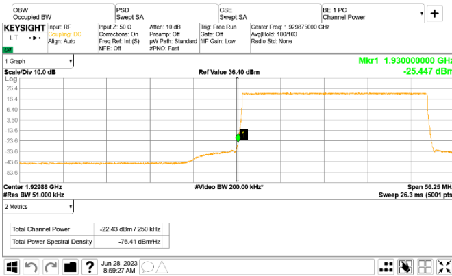
Figure 8.5-155: Conducted emission at the lower band edge
