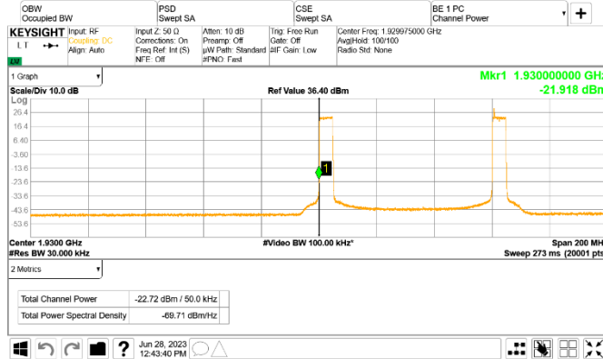
Figure 8.5-179: Conducted emission at the lower band edge
