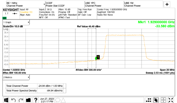
Figure 8.5-140: Conducted emission 1 MHz away from the lower band edge
