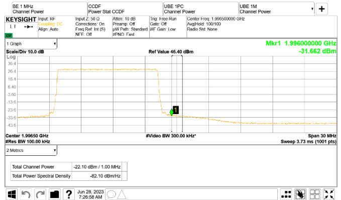
Figure 8.5-146: Conducted emission 1 MHz away from the upper band edge
