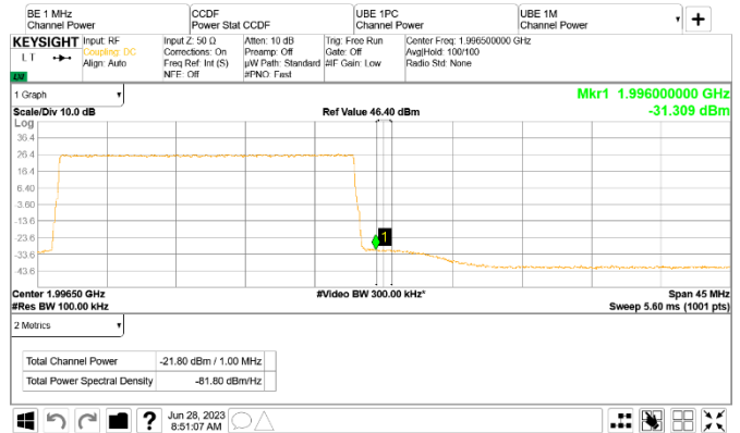
Figure 8.5-154: Conducted emission 1 MHz away from the upper band edge
