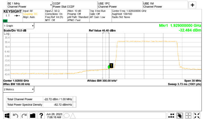
Figure 8.5-144: Conducted emission 1 MHz away from the lower band edge
