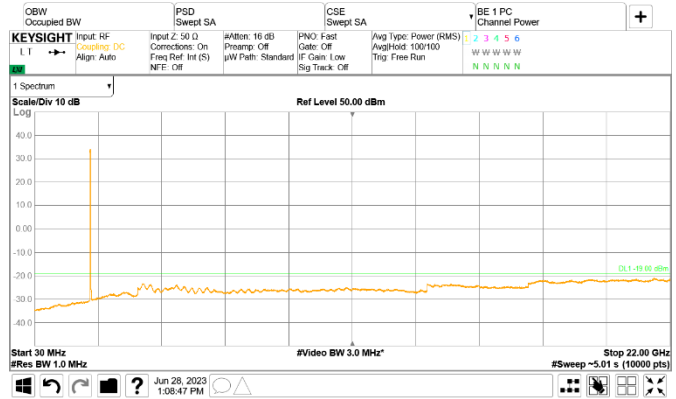
Figure 8.5-84: Conducted spurious emissions of multi-RAT operation, 3 x NR 5 MHz + 3 x LTE with IoT1 5 MHz, Low Channel
