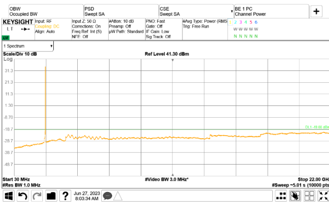
Figure 8.3-57: Conducted spurious emissions of NR 25 MHz top channel, single-carrier operation
