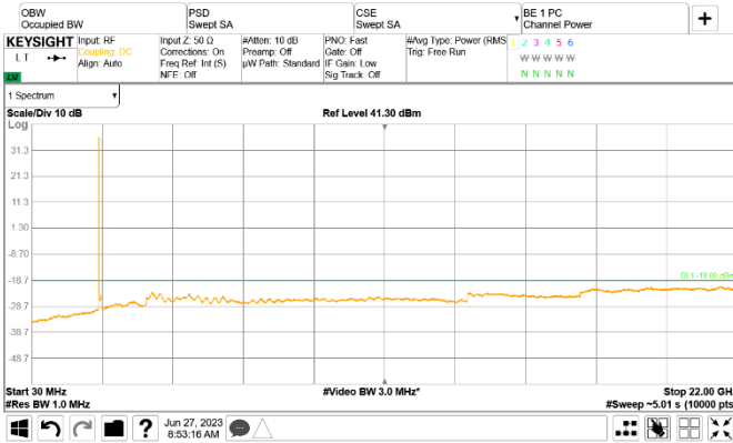
Figure 8.3-33: Conducted spurious emissions of LTE 5 MHz three non-contiguous channels, three-carrier operation
