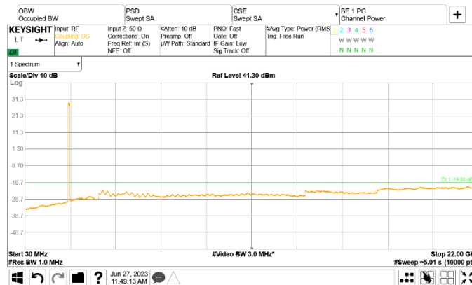
Figure 8.3-78: Conducted spurious emissions of NR 15 MHz six contiguous channels, six-carrier operation
