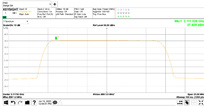
Figure 8.1-7: PSD of LTE 15 MHz channel bandwidth with IoT, single carrier operation, sample plot
