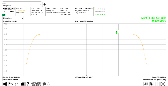
Figure 8.2-16: PSD of NR 20 MHz channel bandwidth, single carrier operation, sample plot
