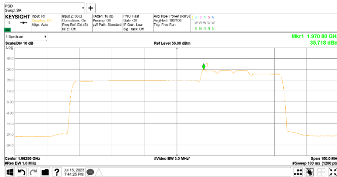
Figure 8.2-31: PSD of multi-RAT operation, NR 40 MHz + 3 × LTE 5 MHz + NR 10 MHz, Low Channel
