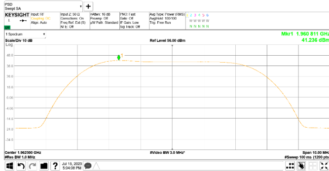
Figure 8.2-5: PSD of LTE 5 MHz channel bandwidth with guard-band, single carrier operation, sample plot
