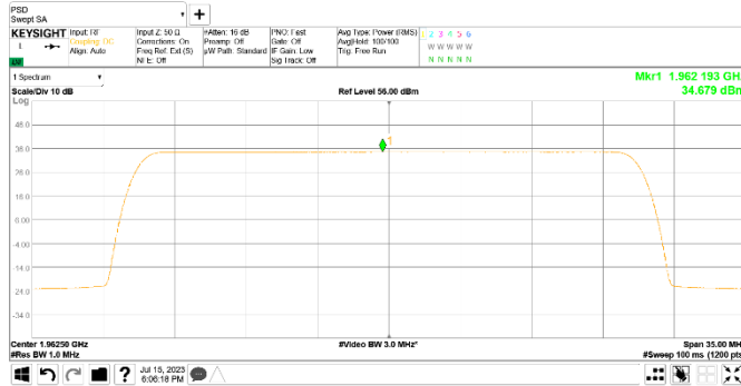
Figure 8.2-17: PSD of NR 25 MHz channel bandwidth, single carrier operation, sample plot
