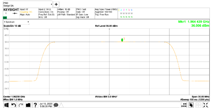
Figure 8.2-4: PSD of LTE 20 MHz channel bandwidth, single carrier operation, sample plot
