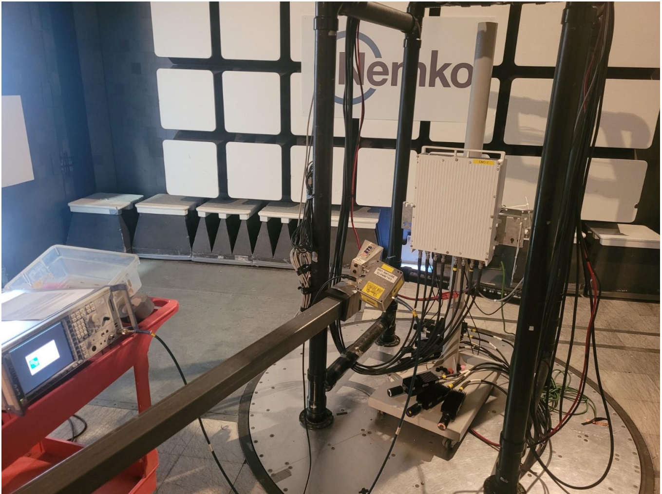
Figure 3.5-6: EUT Set-up photo for Radiated Emissions [18-40 GHz]
